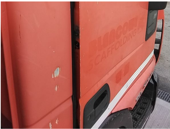
9: Door osf Chipped Edge Chip
