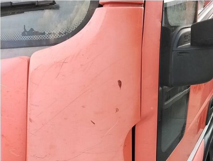
1: Panel Front Scratched Over 25mm Thru Paint
