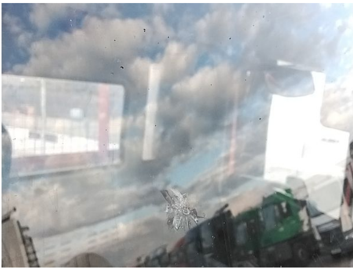
4: Screen Front Chipped UpTo 10mm
