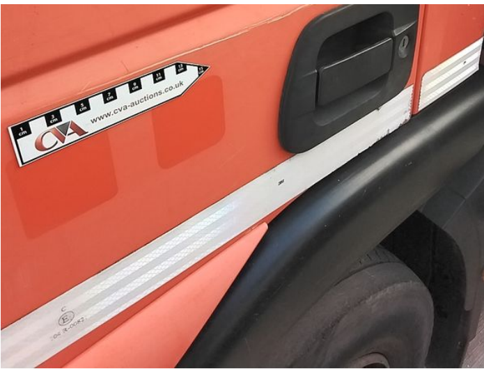
10: Door nsf Scratched Over 25mm Thru Paint
