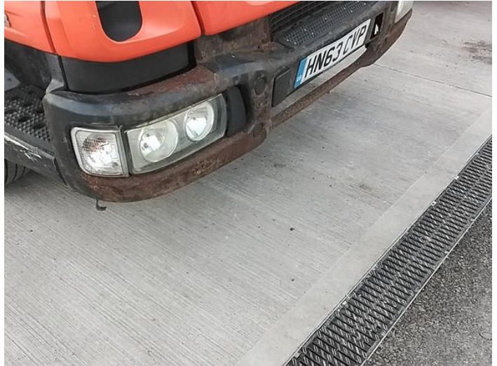
2: Bumper Front Rusted Over 5mm
