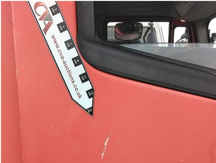
7: Door of Scratched Over 25mm Thru Paint
