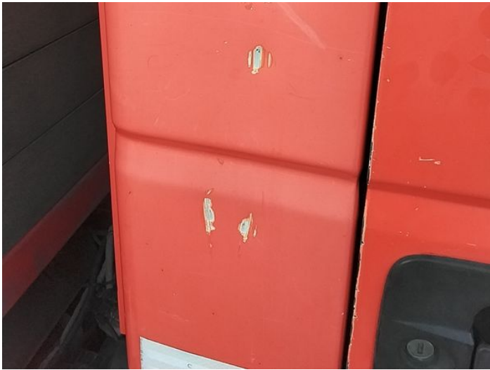
6: Panel Front Dented With Paint Damage
