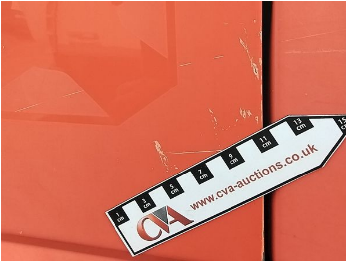
11: Door nsf Scratched Over 25mm Thru Paint
