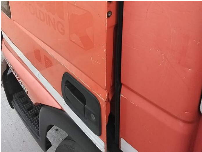
13: Door nsf Chipped Edge Chip
