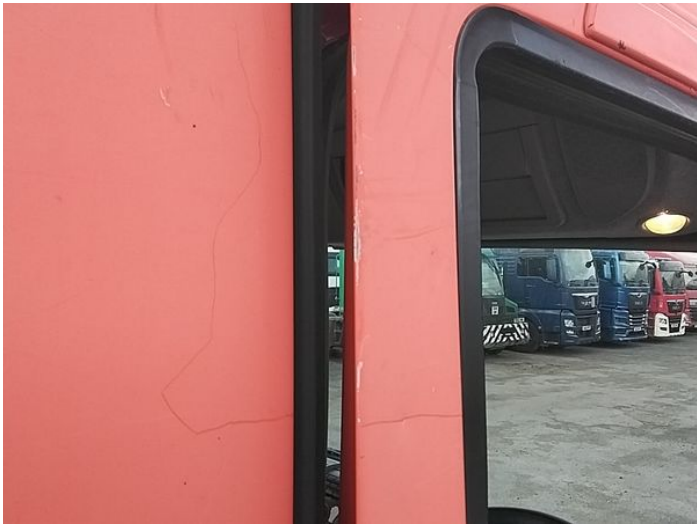
8: Door of Chipped Edge Chip
