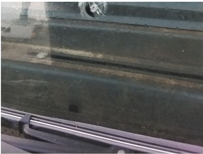
3: Screen Front Chipped UpTo 10mm
