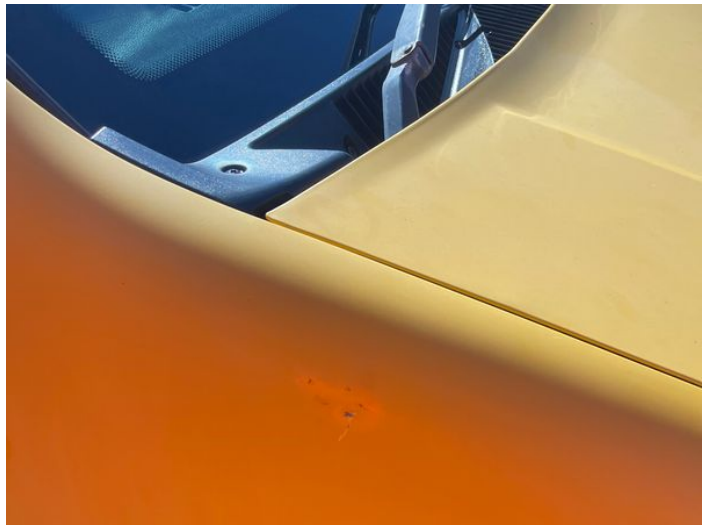
2: Panel Front Dented With Paint Damage
