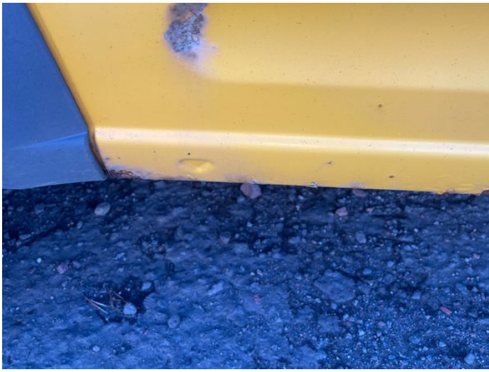
4: Qtr Panel osr Rusted Over 5mm
