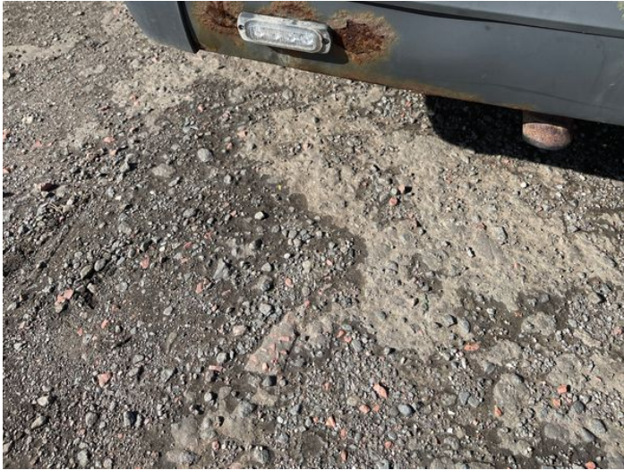
5: Bumper Rear Rusted Over 5mm
