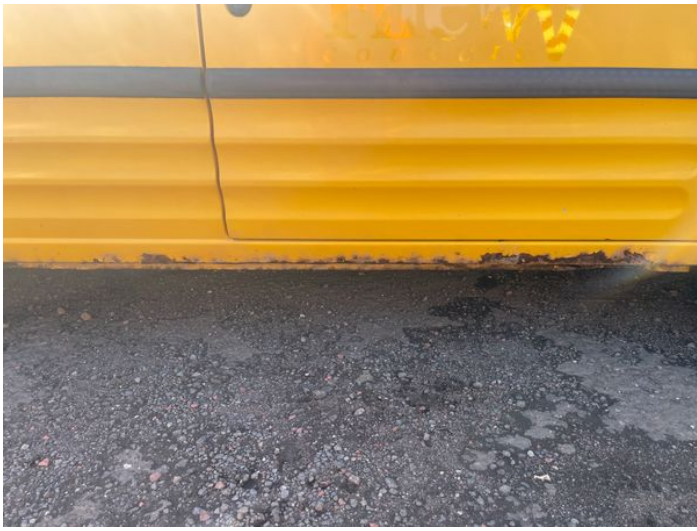
3: Sill os Rusted Over 5mm
