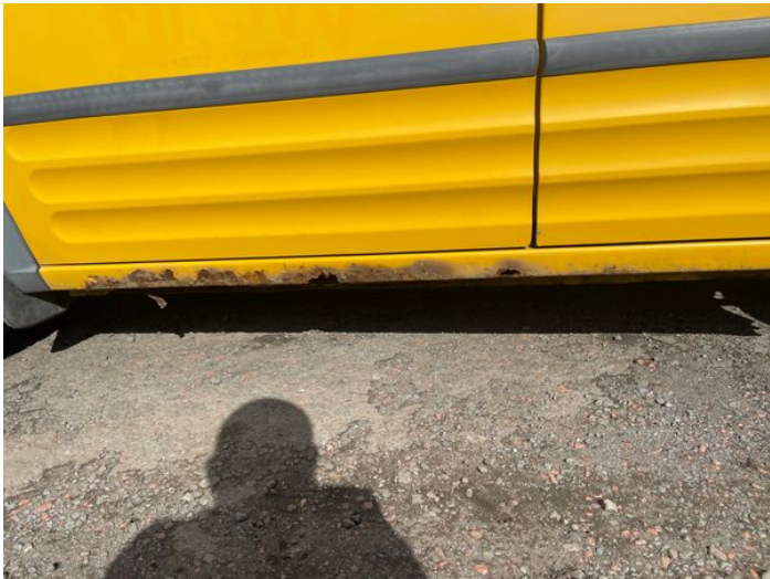
7: Sill ns Rusted Holed
