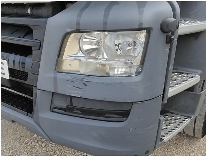
3: Bumper Front Moulding Scuffed (Unpainted) Over 100mm
