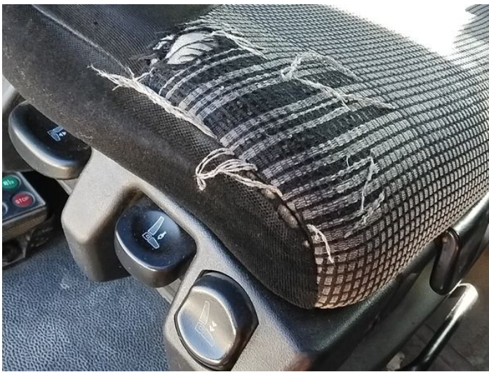
15: Seat Base Cover osf Holed Over 3mm
