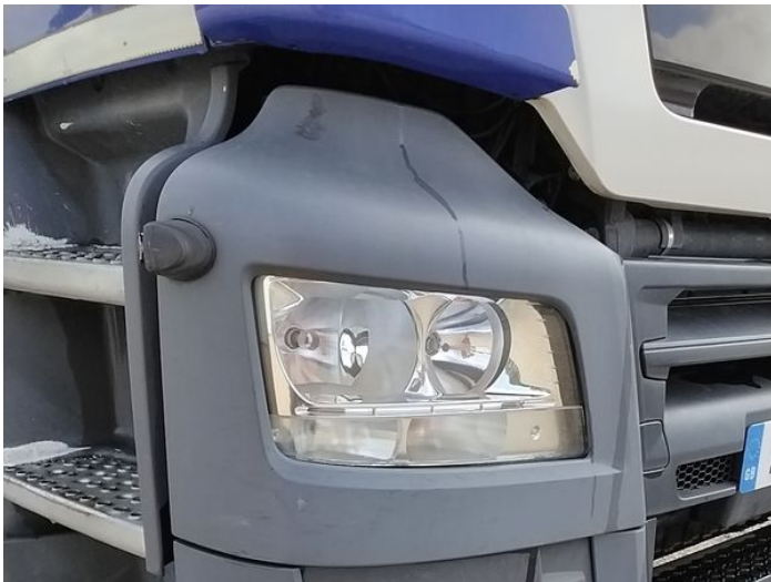
1: Bumper Front Moulding Scuffed (Unpainted) Over 100mm
