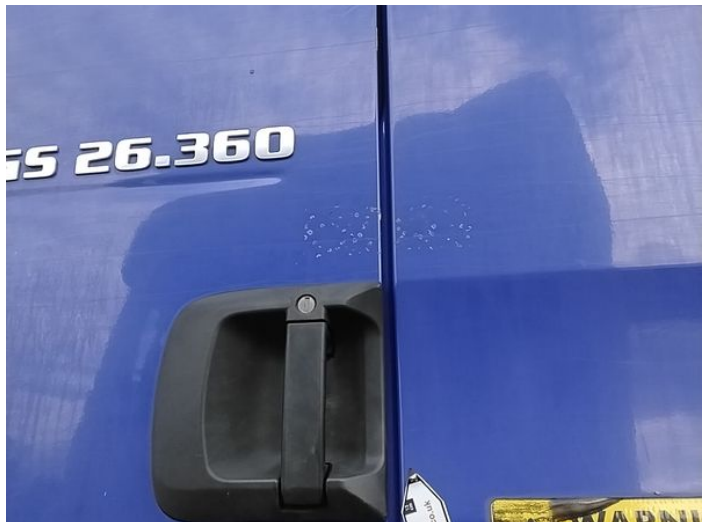
8: Door nsf Chipped Edge Chip
