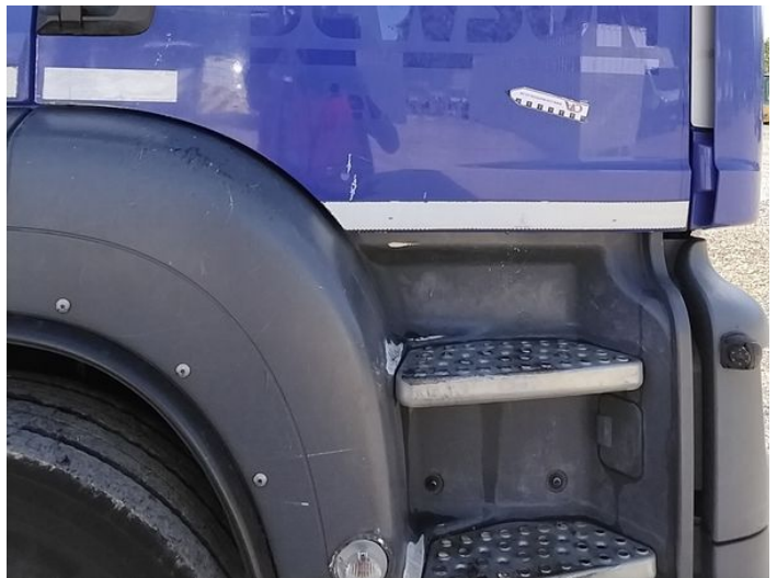
12: Door osf Scratched Over 25mm Thru Paint
