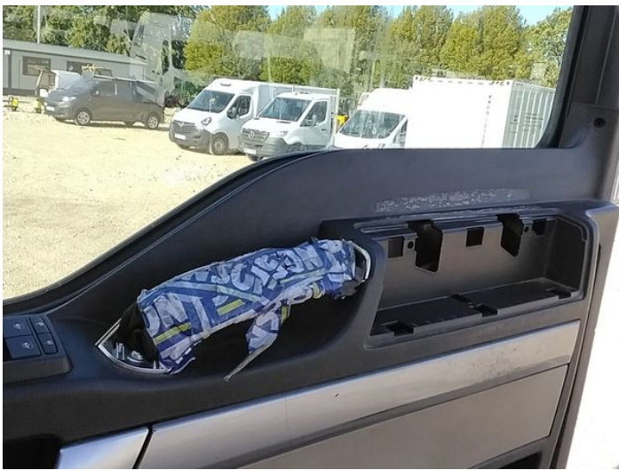
16: Handle Inner osf Damaged Replace
