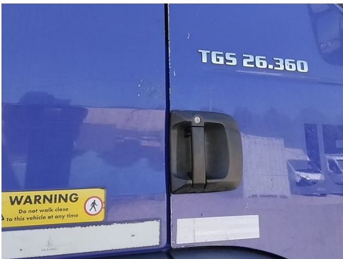
13: Door osf Chipped Edge Chip
