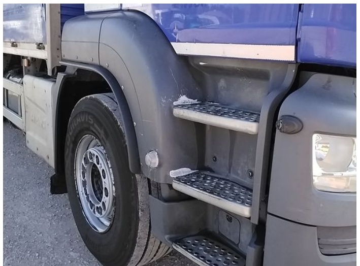
14: Wing Front Arch Extension os Scuffed (Unpainted) Over 100mm
