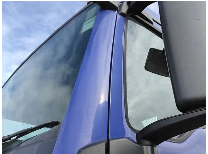
4: A Post ns Scratched Up To 25mm Not Thru Paint
