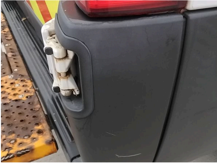
7: Bumper Rear Moulding Scuffed (Unpainted) UpTo 100mm
