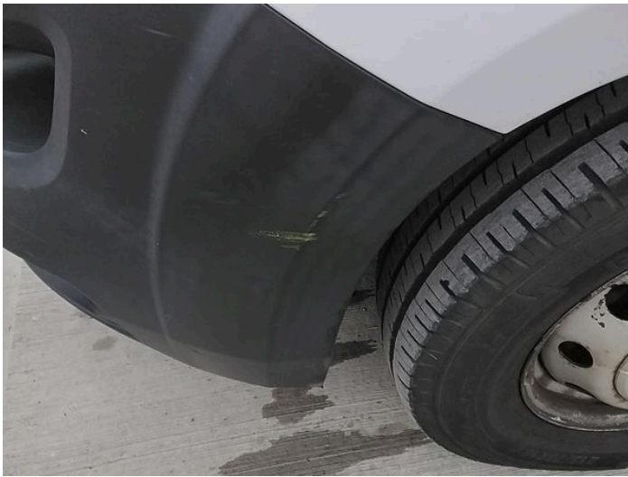
3: Bumper Front Moulding Scuffed (Unpainted) Over 100mm
