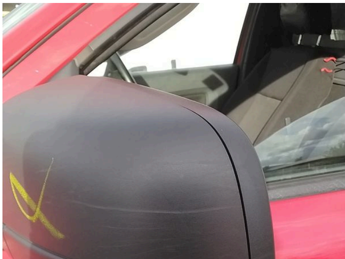
3: Door Mirror Assy nsf Scuffed (Unpainted) Over 100mm
