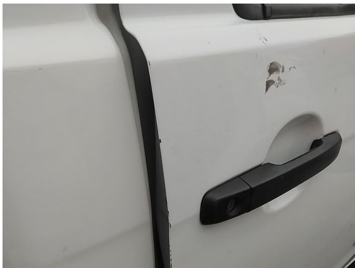
5: Door osf Chipped Edge Chip
