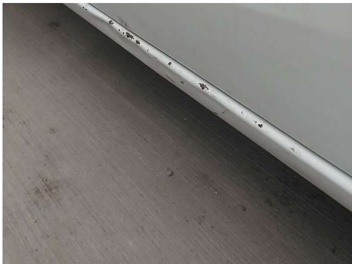
3: Sill os Chipped Multiple Chips
