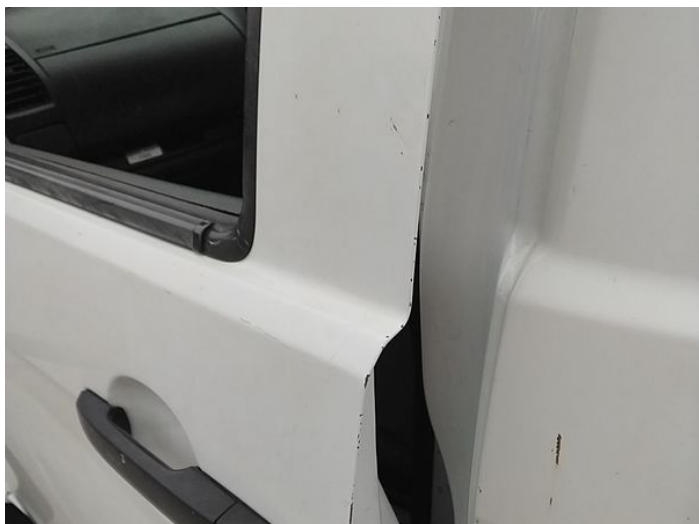
7: Door nsf Chipped Edge Chip
