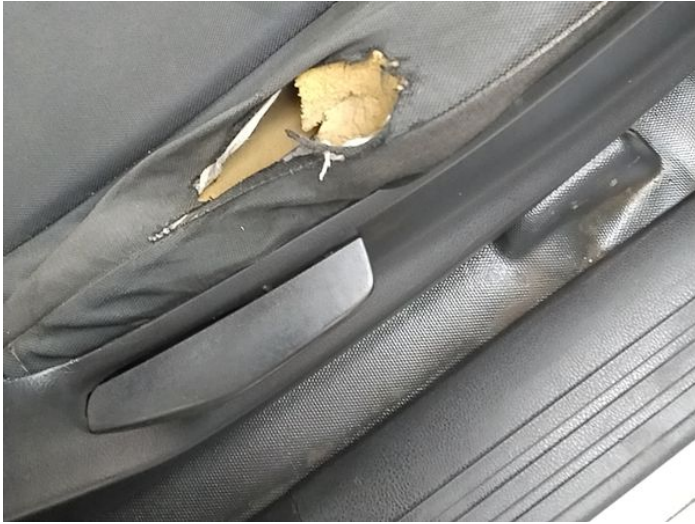
13: Seat Base Cover osf Torn Over 3mm
