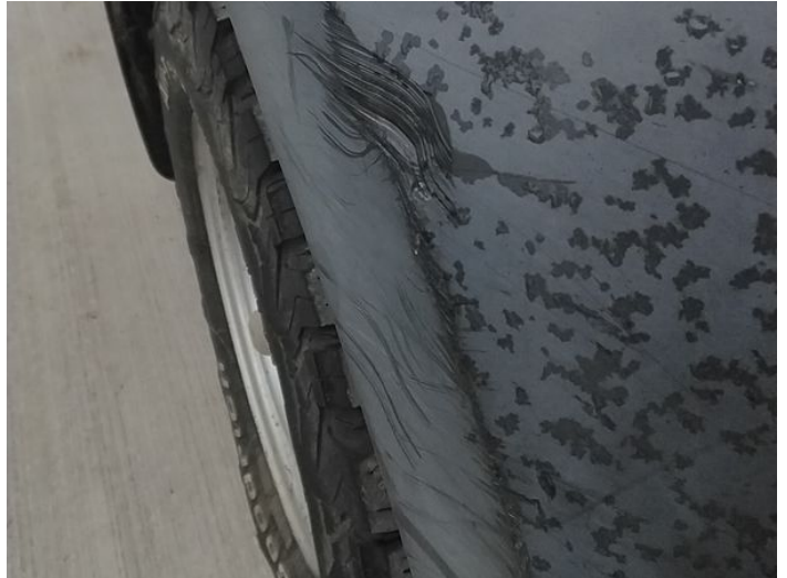
2: Bumper Front Moulding Scuffed (Unpainted) Over 100mm
