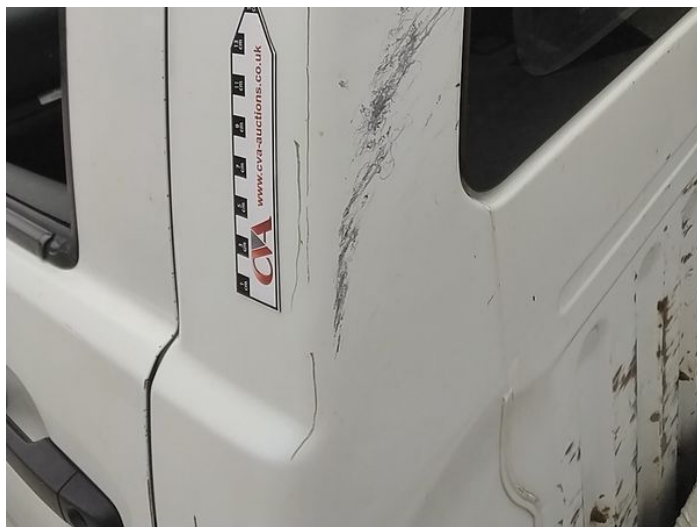
6: C Post ns Scratched Over 25mm Thru Paint
