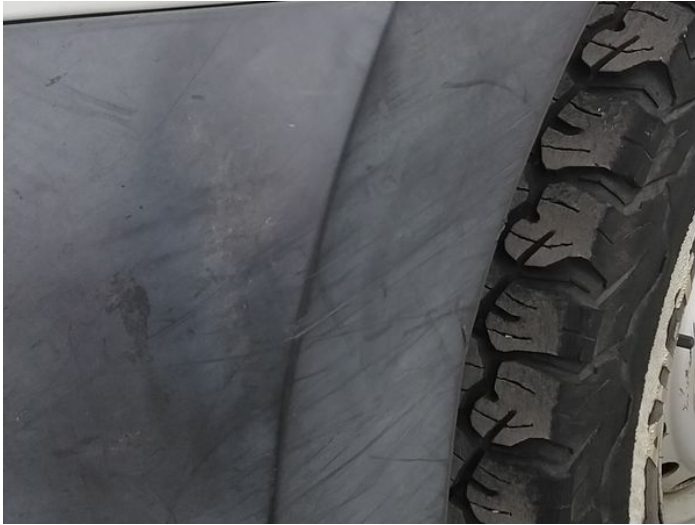
11: Bumper Front Moulding Scuffed (Unpainted) Over 100mm
