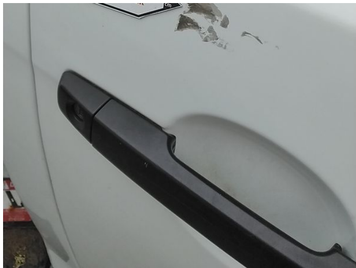
4: Door osf Scratched Over 25mm Thru Paint
