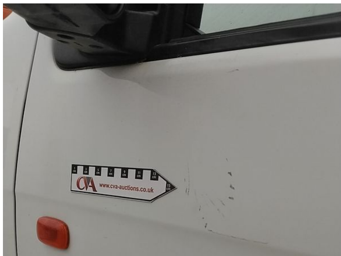
8: Door nsf Scratched Over 25mm Thru Paint
