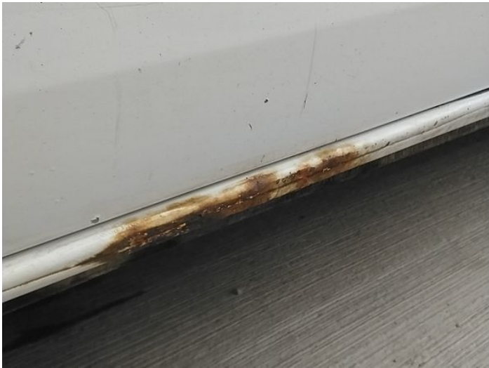
7: Sill ns Rusted Over 5mm
