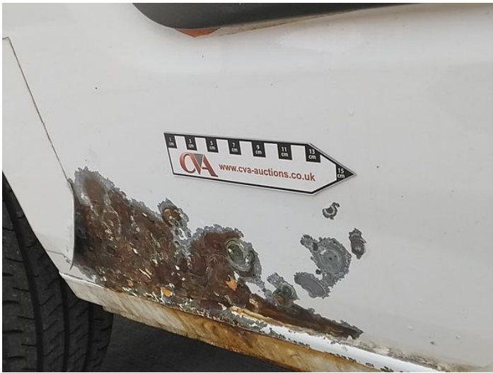
4: Sill os Scratched Rusted
