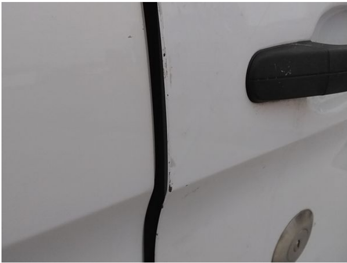
3: Door osf Chipped Edge Chip
