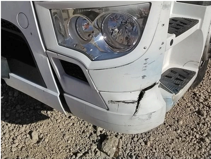
7: Fog Lamp Surrounds Scratched (Painted) Over 25mm Thru Paint
