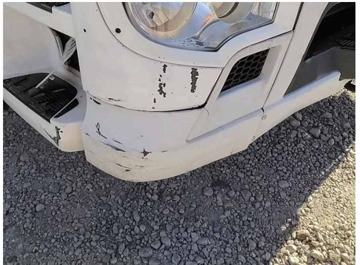
2: Fog Lamp Surround os Scratched (Painted) Over 25mm Thru Paint
