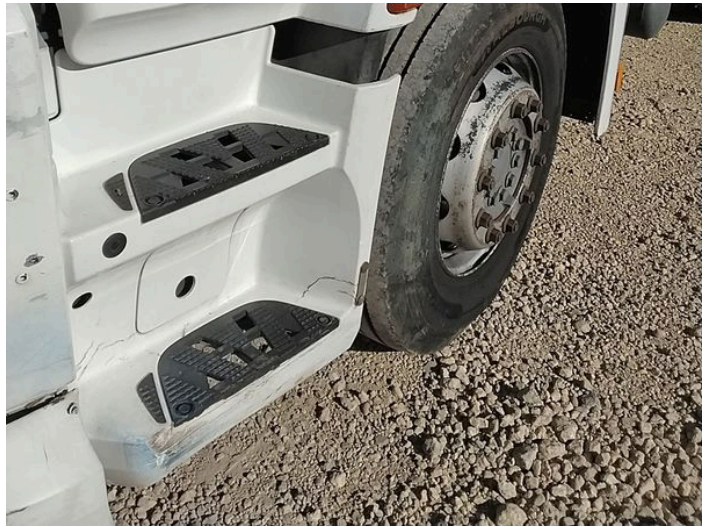
12: Wing Front Arch Extension ns Broken Replace
