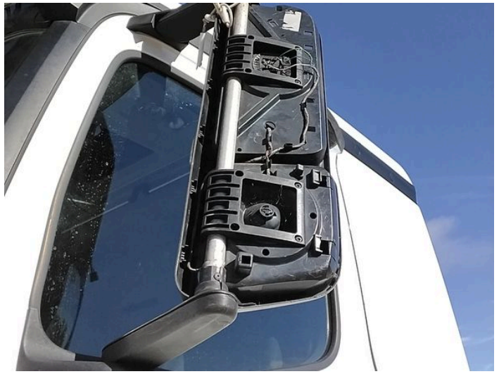
10: Door Mirror Assy nsf Broken Replace
