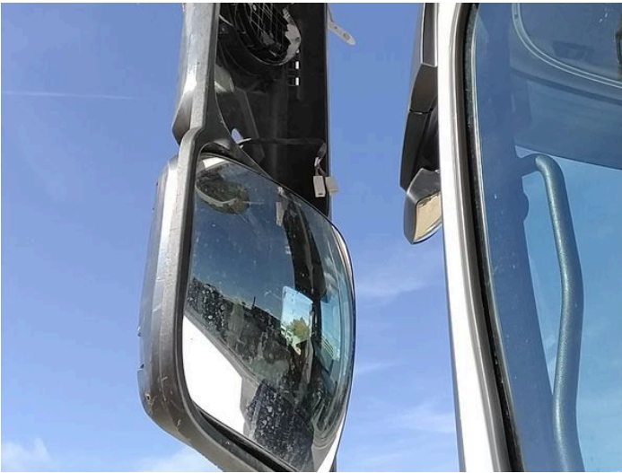
11: Door Mirror Glass ns Missing Replace
