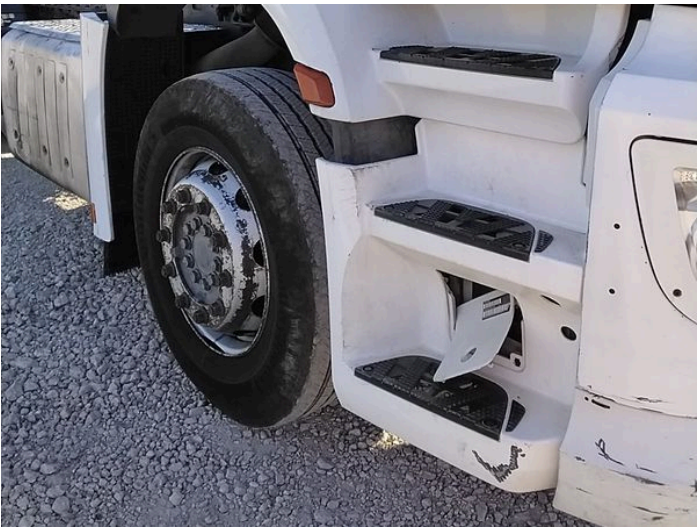
16: Wing Front Arch Extension os Scratched (Painted) Over 25mm Thru Paint
