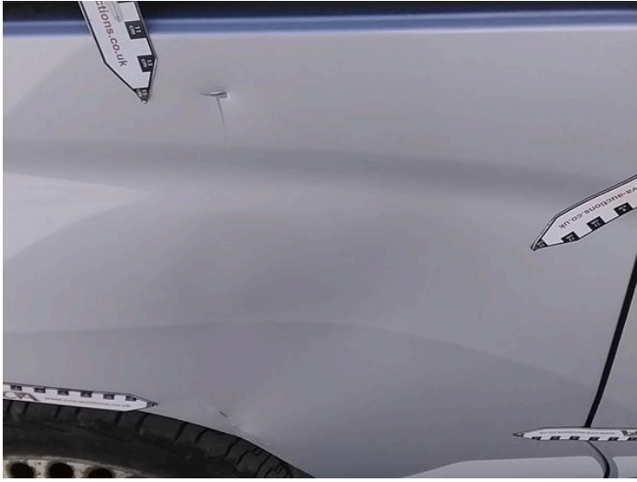
6: Qtr Panel osr Dented With Paint Damage
