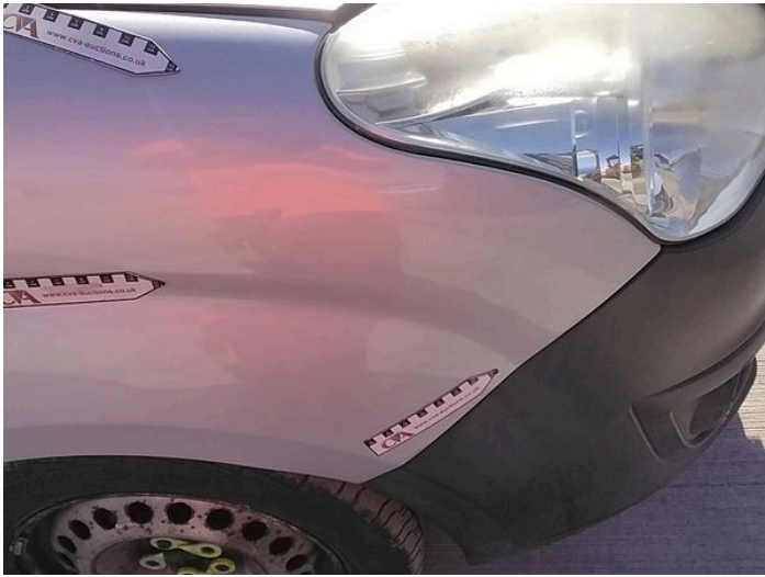
7: Wing osf Dented Over 30mm
