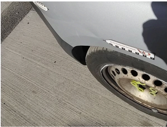
3: Wing nsf Dented Over 30mm
