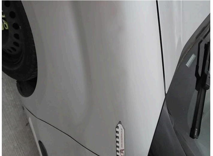
2: Wing nsf Dented Over 30mm
