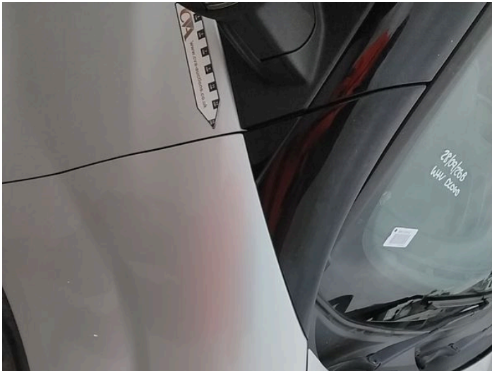
5: Wing osf Scratched Over 25mm Thru Paint
