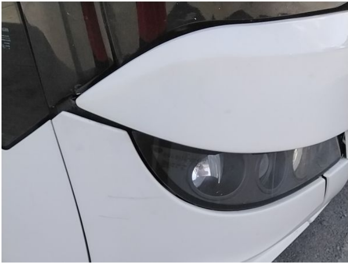
11: Panel Front Scratched Over 25mm Thru Paint
