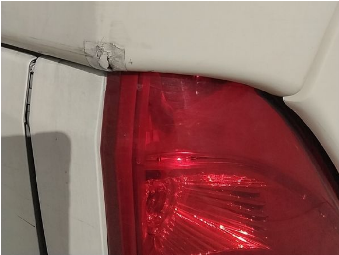
8: Panel Rear Cracked Replace
