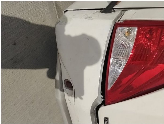
9: Bumper Rear Poor Previous Repair Rippled Over 30%
