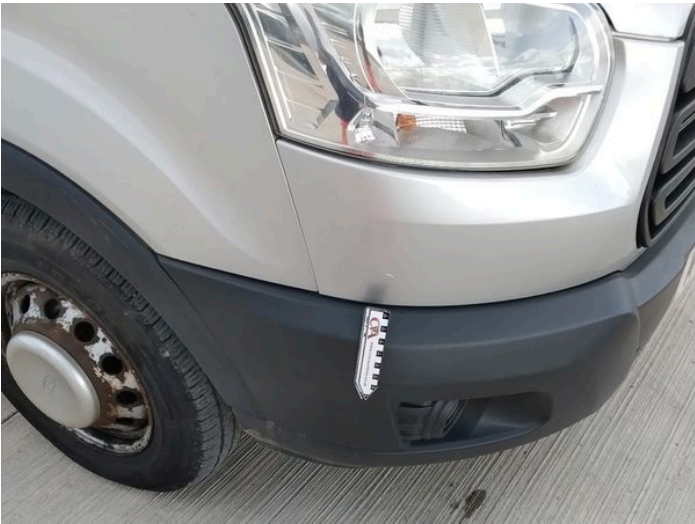
20: Bumper Front Scratched Over 25mm Not Thru Paint
