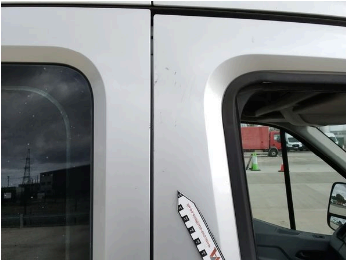
12: Door osf Scratched Over 25mm Thru Paint
