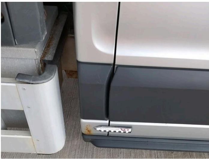
10: Qtr Panel osr Rusted Over 5mm
