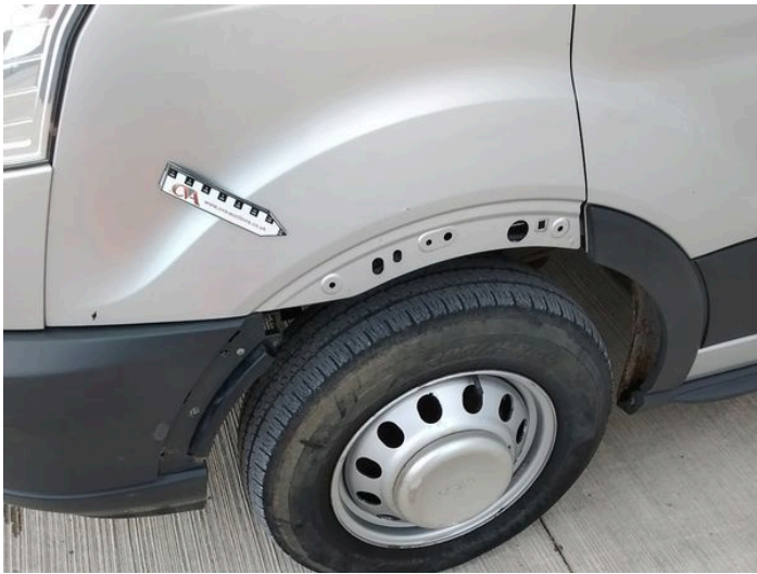
4: Wing Front Arch Extension ns Missing Replace
