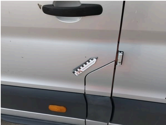
6: Door nsf Chipped Over 5mm
