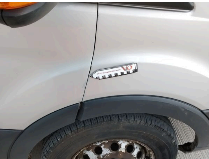
16: Door osf Chipped Over 5mm
