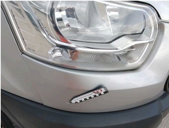
19: Moulding osf Wing Scratched (Painted) Over 25mm Thru Paint
