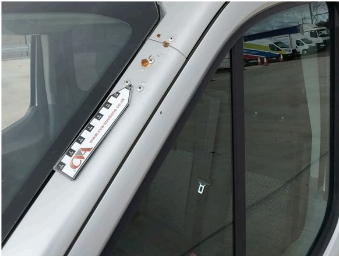
5: A Post ns Rusted Over 5mm
