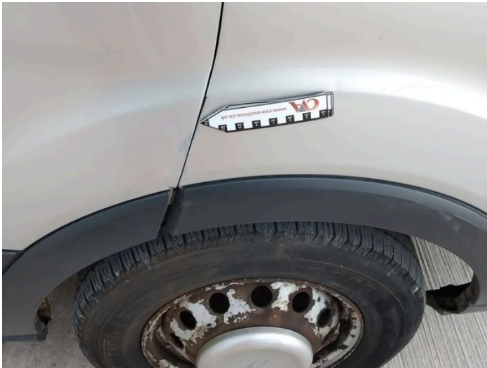
17: Wing osf Chipped Over 5mm
