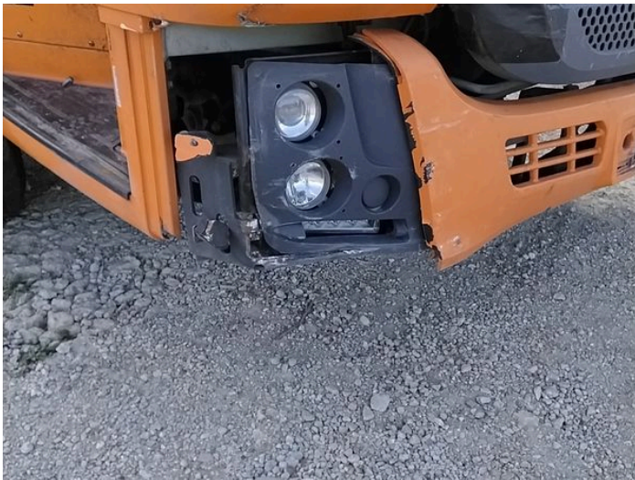
1: Bumper Front Missing Replace
