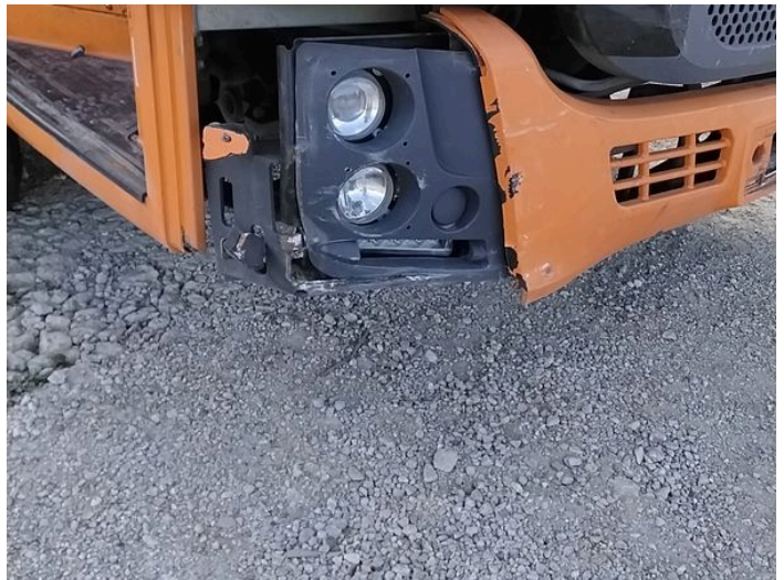
2: Fog Lamp Surround is Broken Replace
