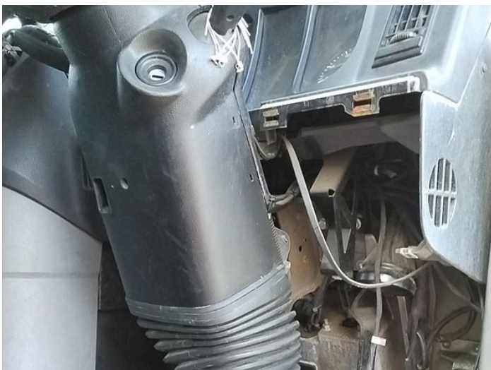
19: Switches And Controls Missing Replace
