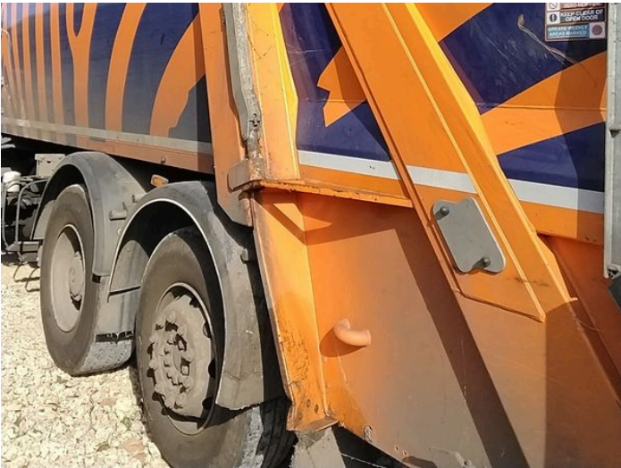
13: Qtr Panel nsr Scratched Over 25mm Thru Paint
