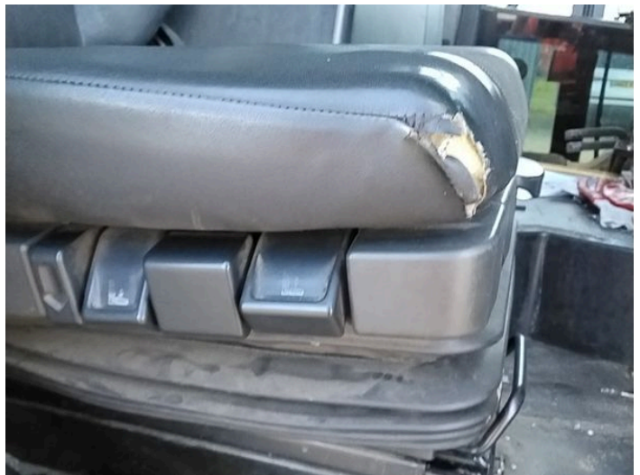
18: Seat Base Cover osf Holed Over 3mm
