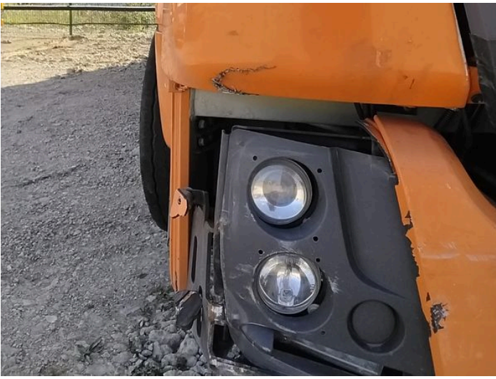
9: Wing nsf Cracked Replace
