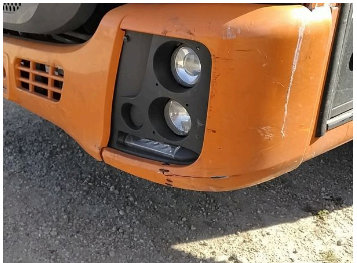
8: Bumper Front Cracked Over 25mm
