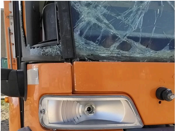
23: Flasher Side Repeater os Broken Replace
