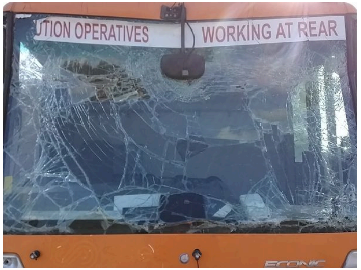
4: Screen Front Cracked Replace
