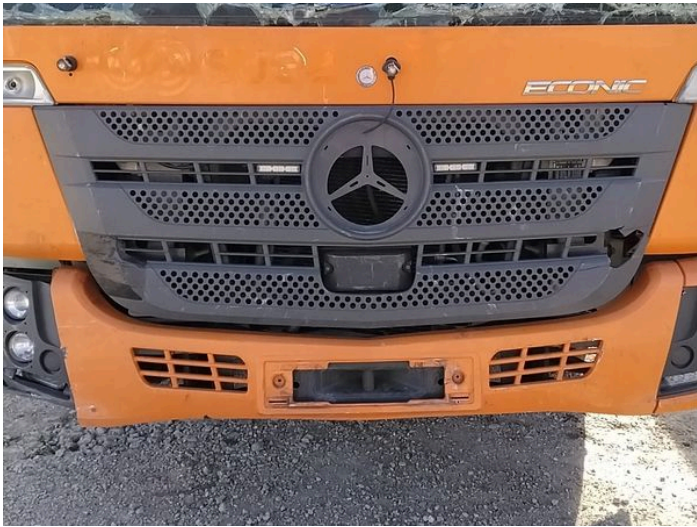
5: Grille Front Broken Replace
