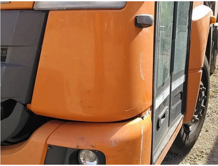
10: Wing nsf Scratched Over 25mm Not Thru Paint
