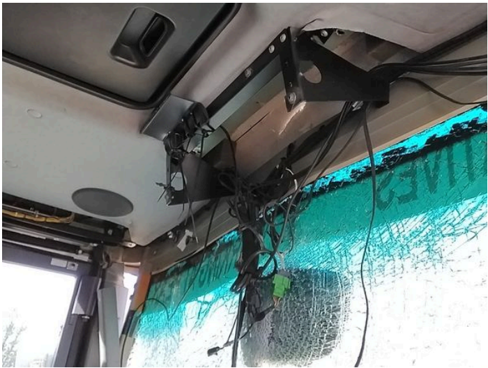
22: Switches And Controls Missing Replace
