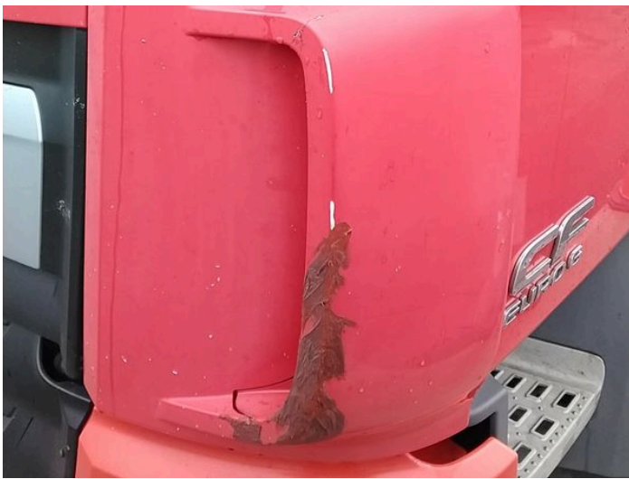
3: Panel Front Cracked Replace
