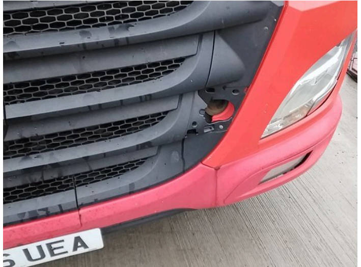
2: Bumper Front Moulding Missing Replace
