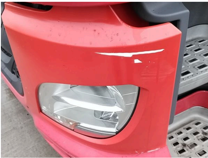
4: Panel Front Scratched Over 25mm Thru Paint
