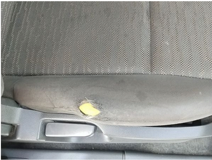
16: Seat Base Cover osf Holed Over 3mm
