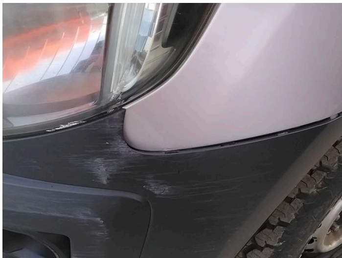
3: Bumper Front Scratched Over 100mm Thru Paint
