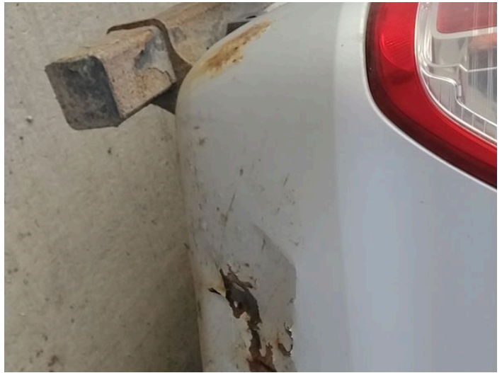
12: Qtr Panel osr Rusted Holed
