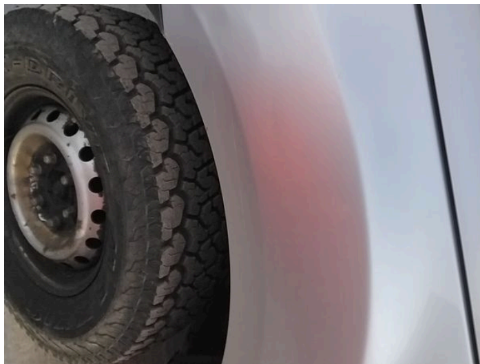
4: Wing nsf Dented With Paint Damage
