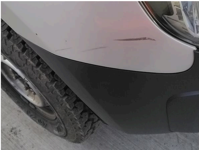
1: Wing of Scratched Over 25mm Thru Paint
