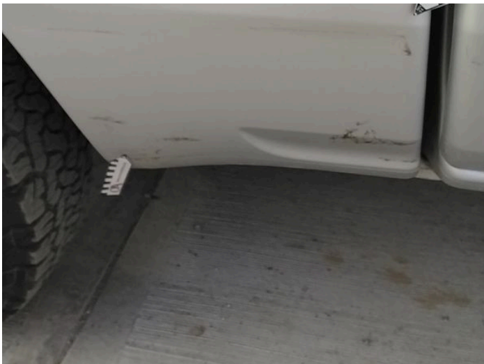
13: Qtr Panel osr Scratched Over 25mm Thru Paint
