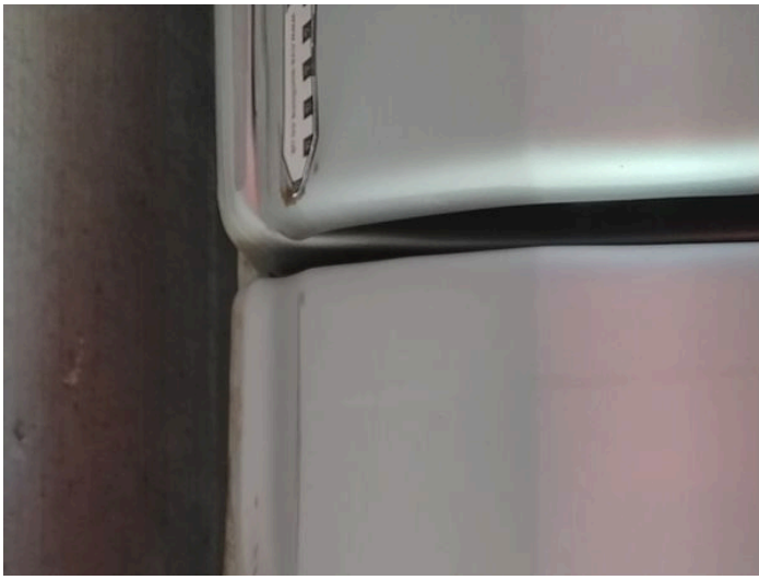
9: Qtr Panel nsr Dented With Paint Damage
