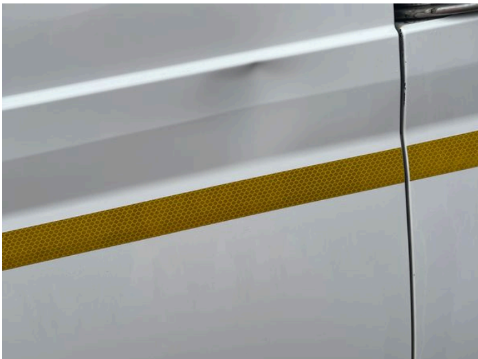
7: Qtr Panel nsr Dented Over 30mm
