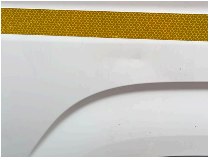
5: Qtr Panel osr Dented Over 30mm
