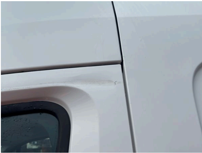
10: Door nsf Dented With Paint Damage
