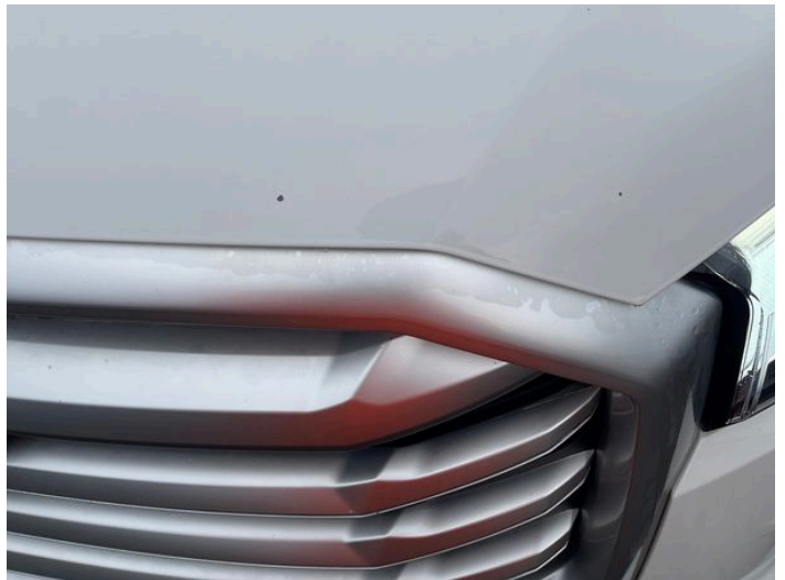
2: Bonnet Chipped Multiple Chips
