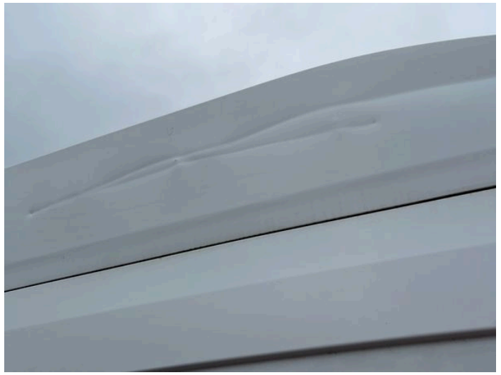
4: Qtr Panel osr Dented With Paint Damage
