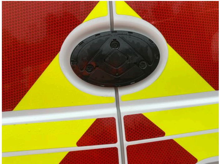
6: Badgedecal Rear Missing Replace
