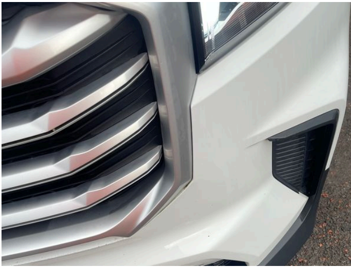
3: Bumper Front Chipped Multiple Chips
