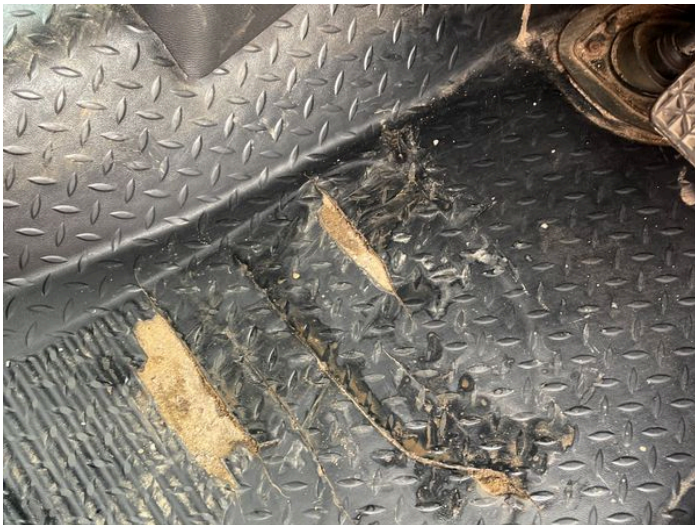
1: Carpets Front Torn Over 10mm
