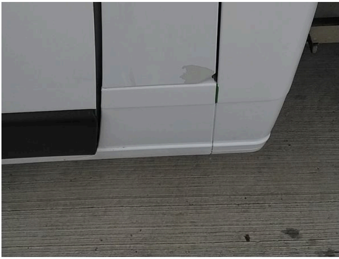
9: Fuel Flap Scratched Over 25mm Thru Paint
