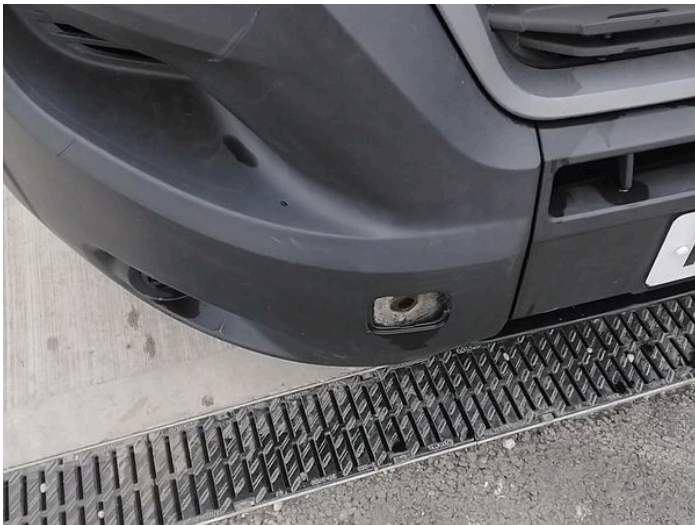
1: Bumper Front Moulding Missing Replace
