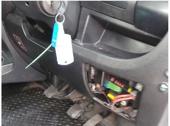
18: Fascia Panel Missing Replace
