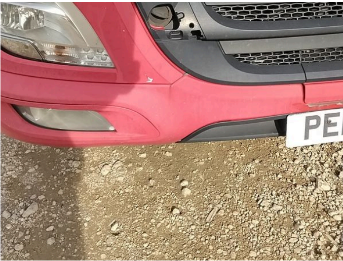
4: Front TowEye Cvr Missing Replace
