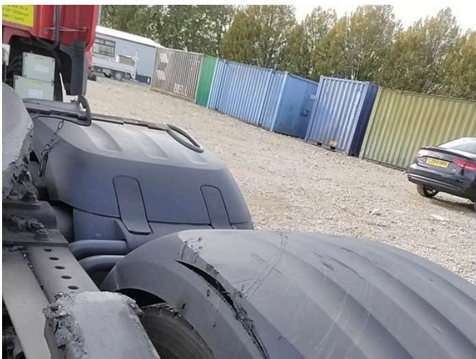
13: Qtr Panel Arch Extension os Broken Replace
