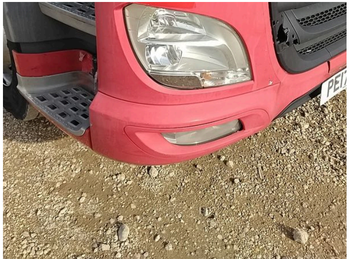
2: Fog Lamp Surround os Broken Replace
