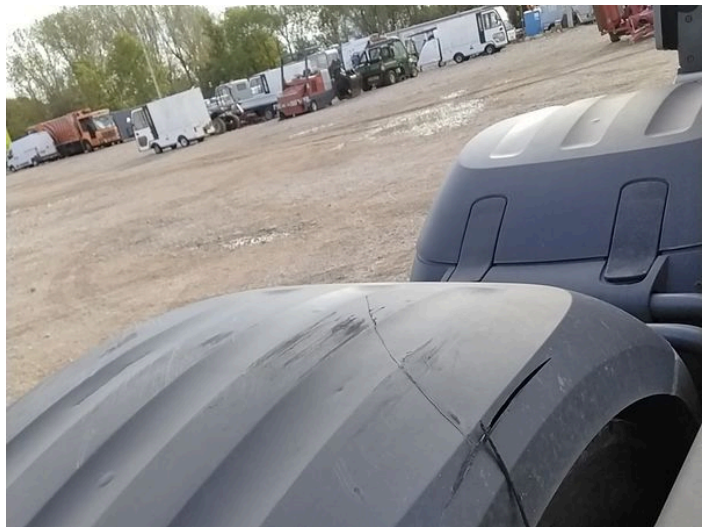
12: Qtr Panel Arch Extension ns Broken Replace
