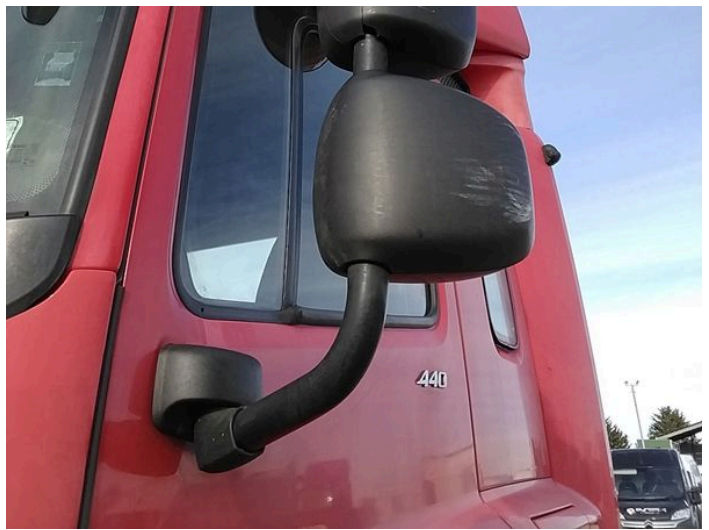
10: Door Mirror Assy nsf Broken Replace
