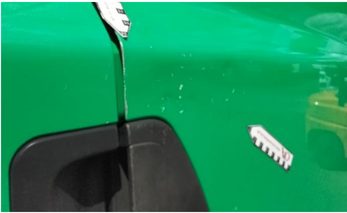
3: Bumper Front Scratched Over 100mm Thru Paint
