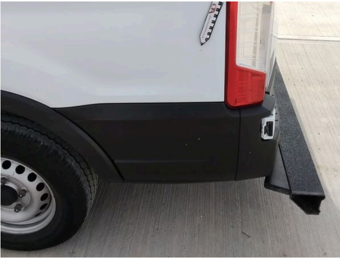
12: Qtr Panel nsr Chipped Over 5mm
