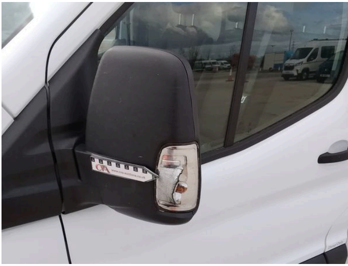
3: Door Mirror Assy nsf Broken Replace
