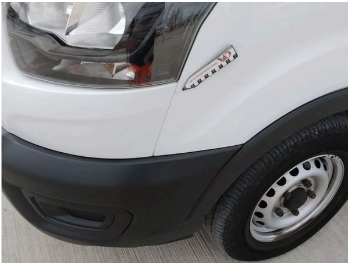
1: Wing nsf Scratched Over 25mm Not Thru Paint
