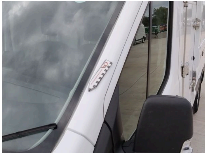
2: A Post ns Chipped Over 5mm
