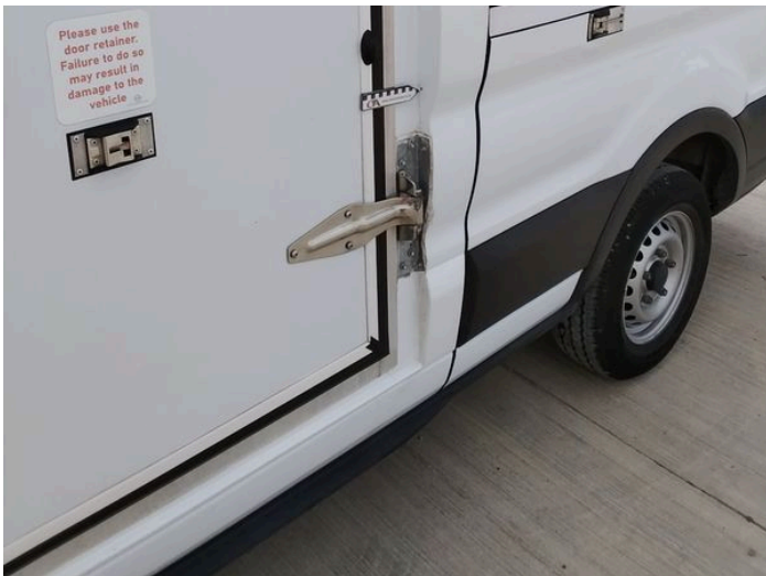
7: Qtr Panel nsr Cracked Replace
