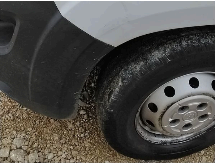
4: Wing nsf Dented With Paint Damage
