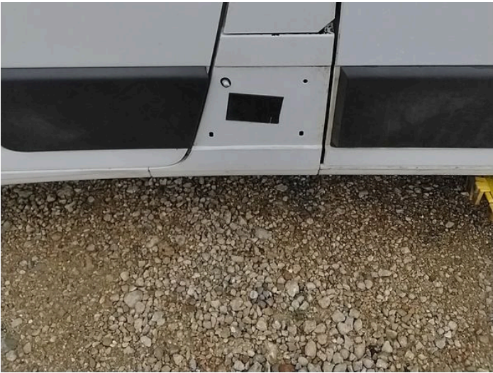
6: Qtr Panel Trim ns Missing Replace
