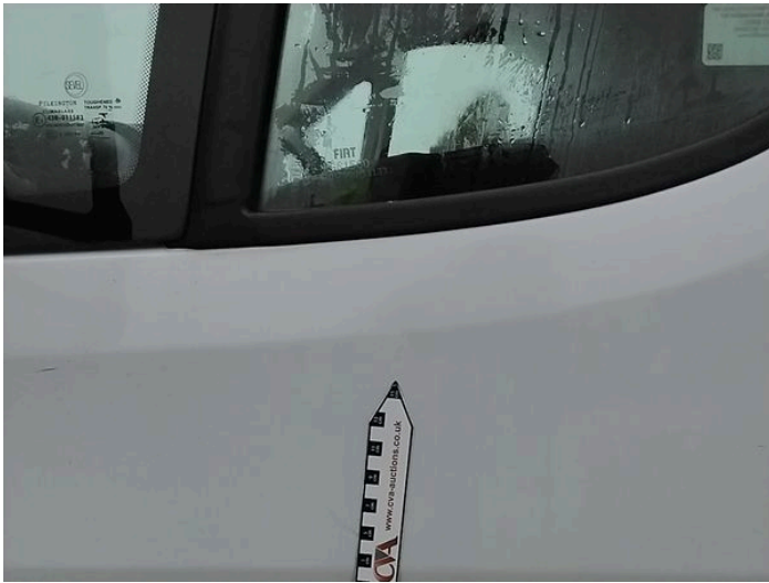
5: Door nsf Dented Over 2 UpTo 10mm
