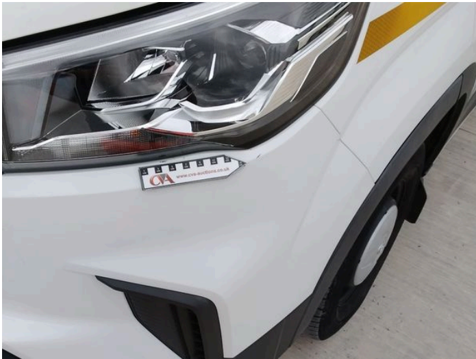
5: Bumper Front Scratched Over 100mm Thru Paint
