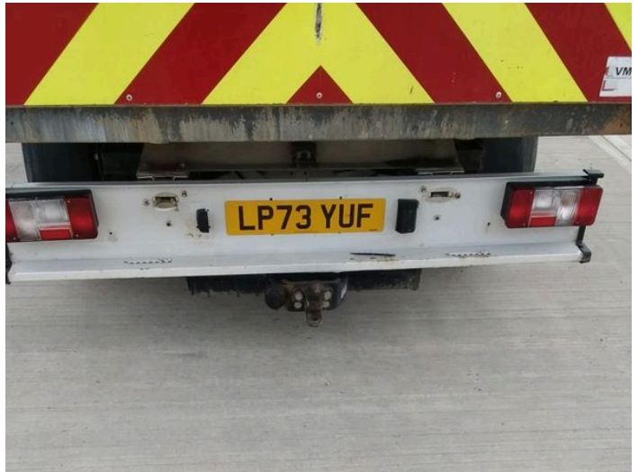
6: Bumper Rear Rusted Over 5mm
