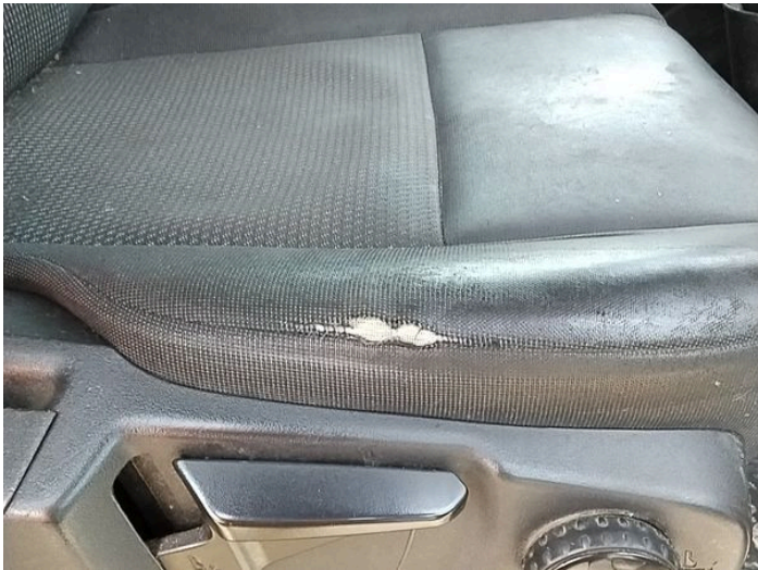
25: Seat Base Cover osf Holed Over 3mm
