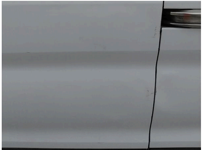
12: Door nsr Dented With Paint Damage
