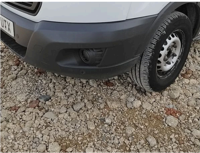
4: Bumper Front Moulding Scuffed (Unpainted) Over 100mm
