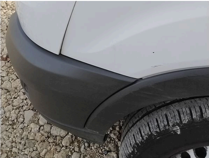
6: Wing nsf Dented Between 10mm + 30mm
