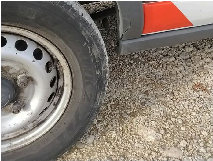
22: Qtr Panel Arch Extension os Broken Replace
