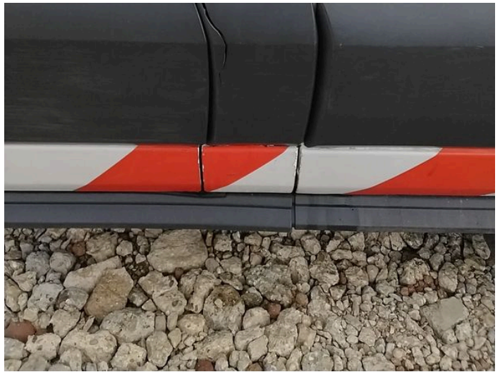
10: Qtr Panel nsr Cracked Replace
