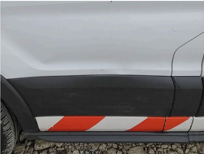
8: Door nsf Dented Over 30mm
