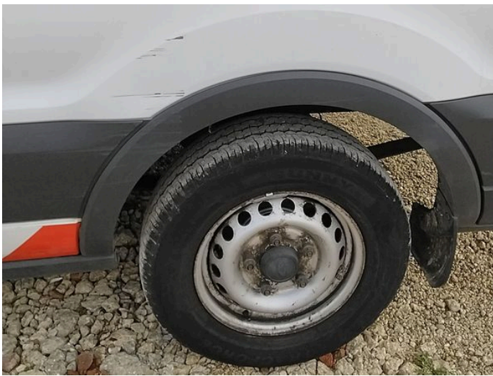
15: Qtr Panel nsr Dented With Paint Damage
