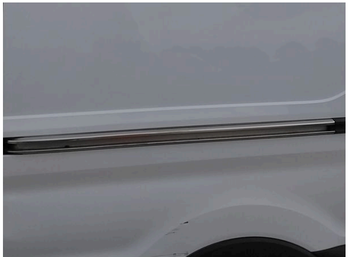
14: Qtr Panel nsr Scratched Over 25mm Not Thru Paint
