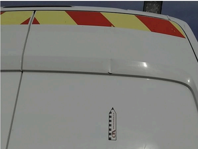
18: Door osr Dented With Paint Damage
