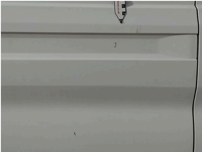
24: Qtr Panel osr Scratched UpTo 25mm Thru Paint
