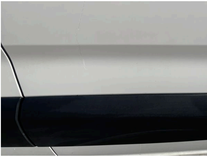
3: Door osf Scratched Over 25mm Thru Paint
