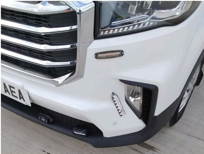
5: Bumper Front Chipped Multiple Chips
