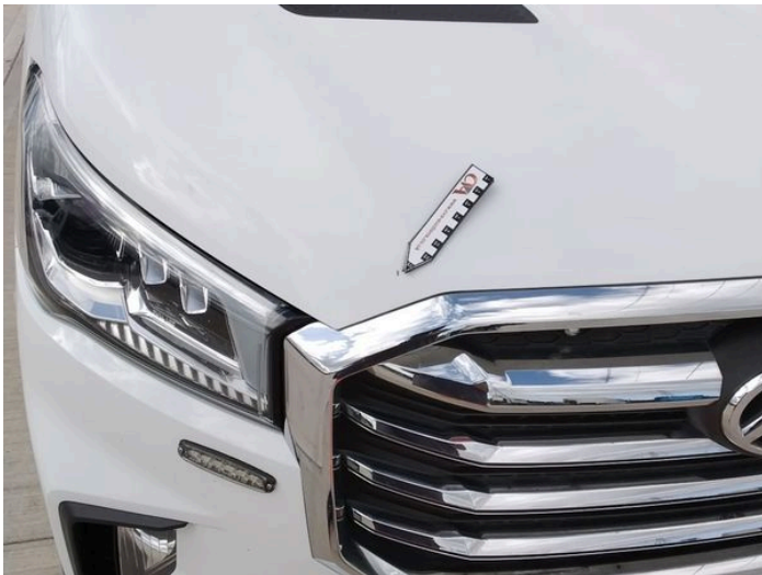
1: Bonnet Chipped Over 5mm
