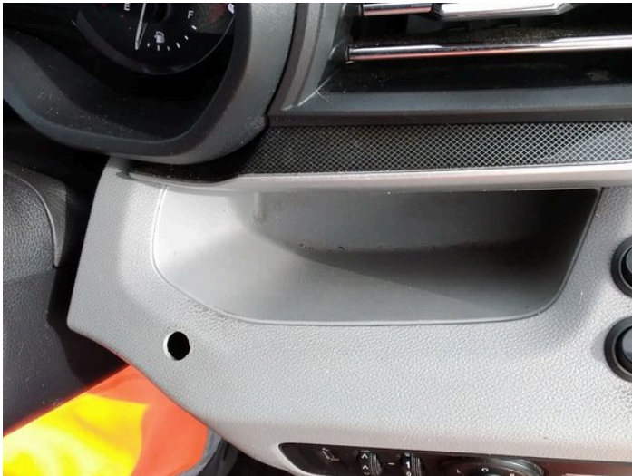
18: Centre Console Front Holed Over 3mm
