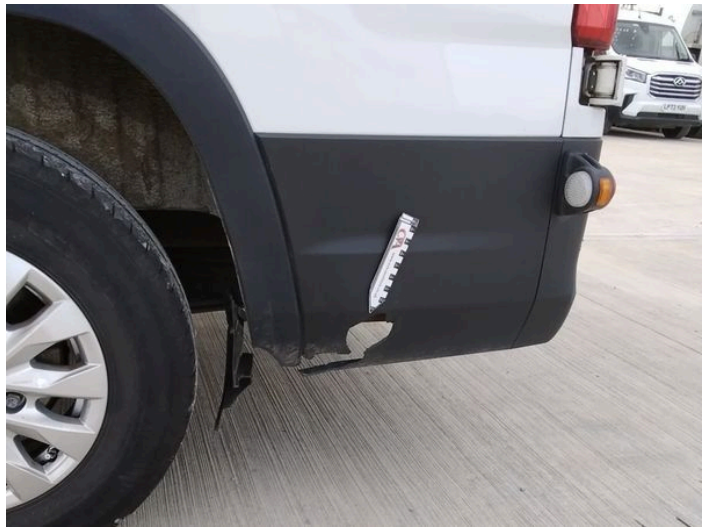
10: Qtr Panel Arch Extension ns Broken Replace
