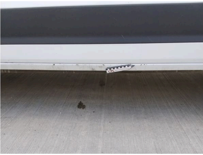
9: Sill ns Chipped Over 5mm
