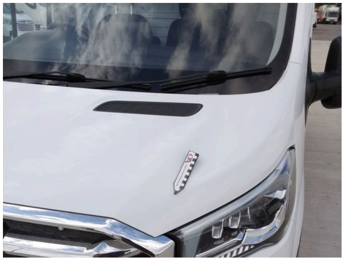
4: Bonnet Chipped Over 5mm
