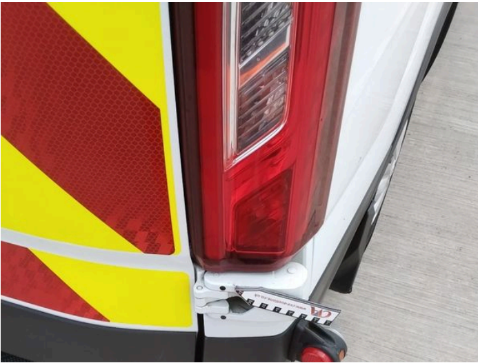
11: Door osr Chipped Over 5mm
