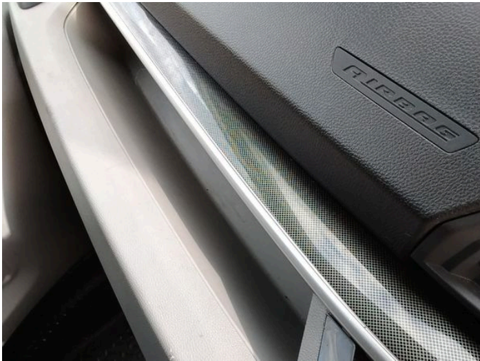
19: Centre Console Front Scuffed Over 25mm
