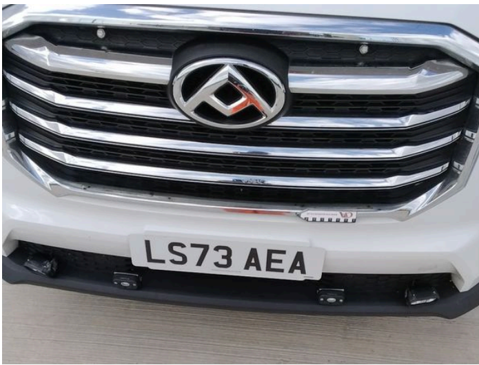
3: Grille Front Scratched (Painted) Over 25mm Not Thru Paint
