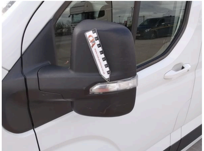
6: Door Mirror Assy nsf Scuffed (Unpainted) Over 100mm
