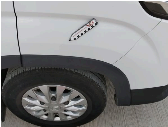
15: Wing osf Scratched Over 25mm Thru Paint
