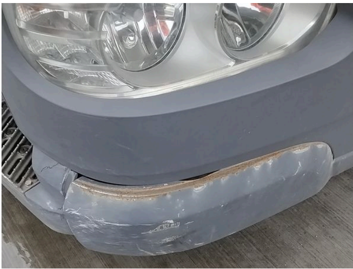
3: Bumper Front Dented With Paint Damage
