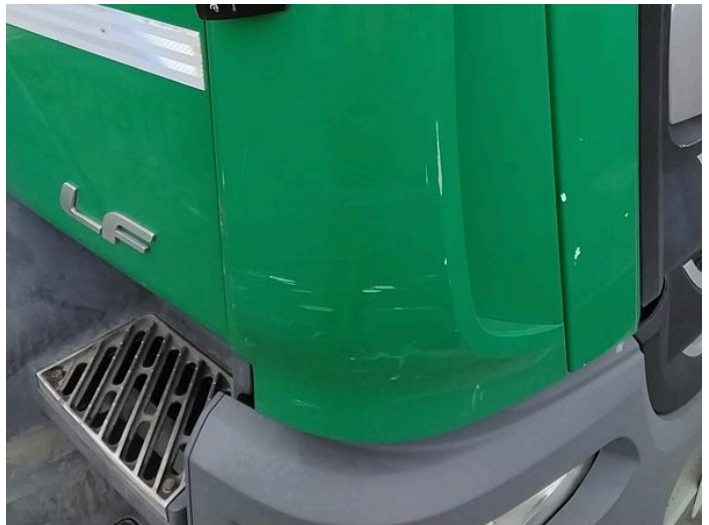
2: Panel Front Scratched Over 25mm Thru Paint
