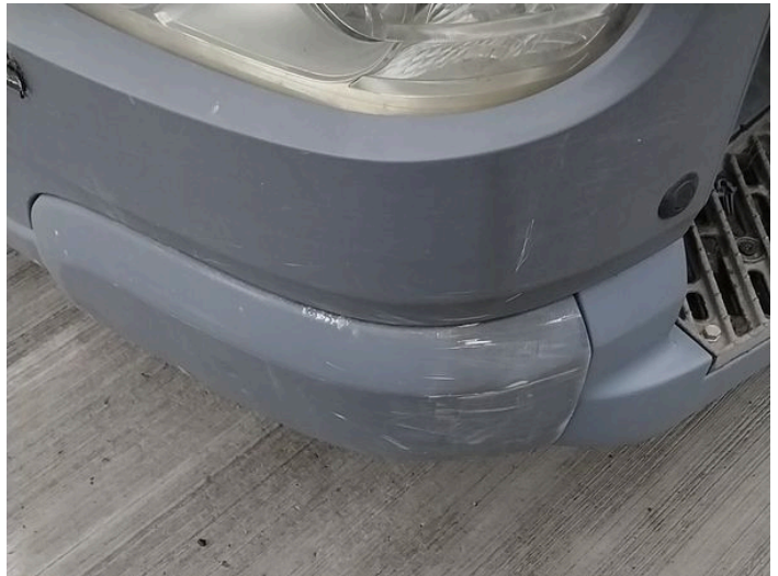
6: Bumper Front Dented With Paint Damage
