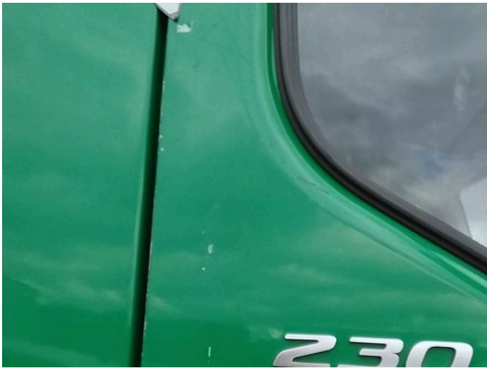
9: Door osf Dented With Paint Damage
