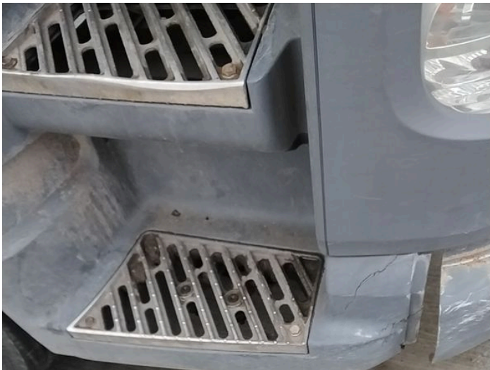
1: Bumper Front Moulding Broken Replace
