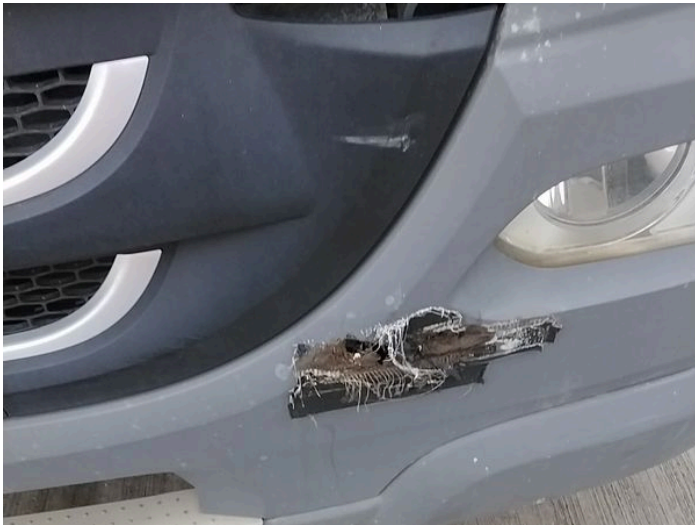
5: Panel Front Cracked Replace
