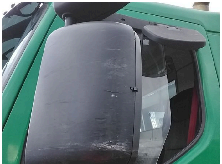
8: Door Mirror Assy nsf Broken Replace
