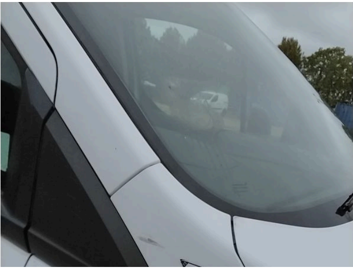
3: A Post os Scratched UpTo 25mm Not Thru Paint
