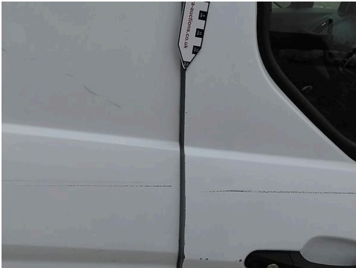
12: Door osf Chipped Edge Chip
