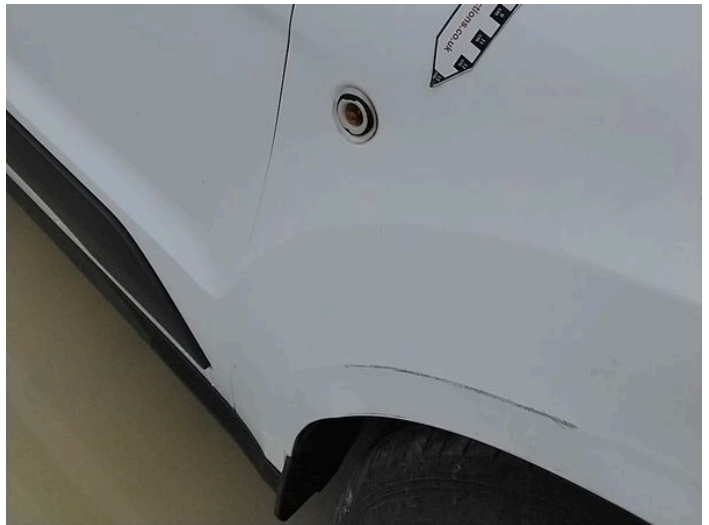
2: Flasher Side Repeater os Broken Replace
