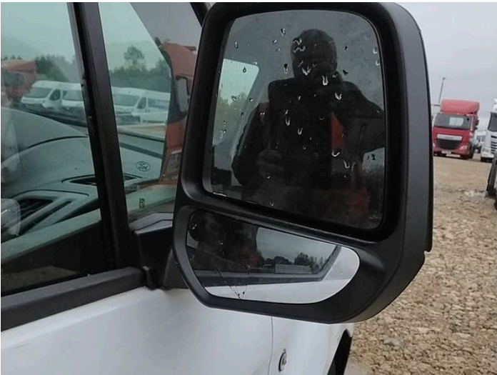
11: Door Mirror Glass os Broken Replace
