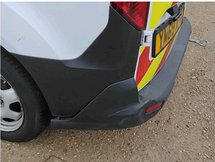
7: Bumper Rear Moulding Broken Replace
