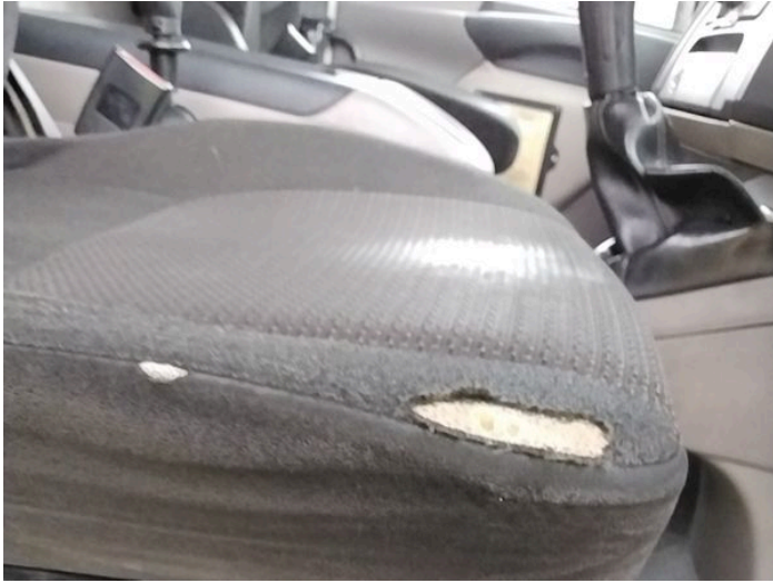
13: Seat Base Cover osf Holed Over 3mm
