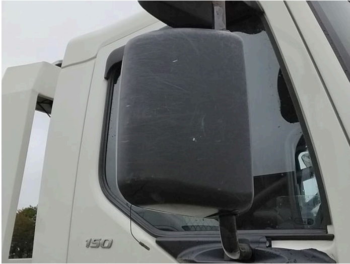
11: Door Mirror Assy osf Broken Replace
