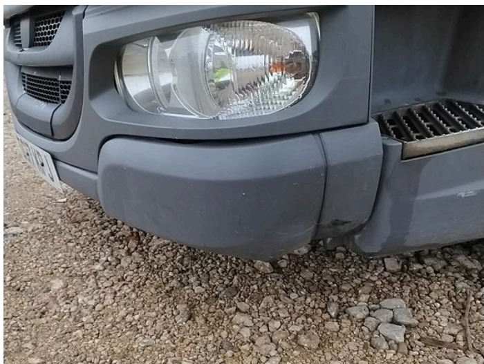
5: Bumper Front Dented Between 10mm + 30mm
