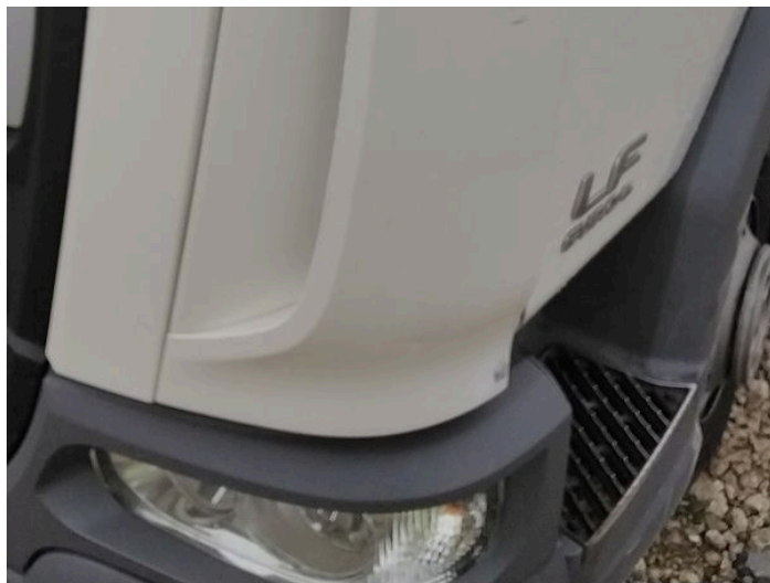
4: Wing nsf Scratched Over 25mm Thru Paint
