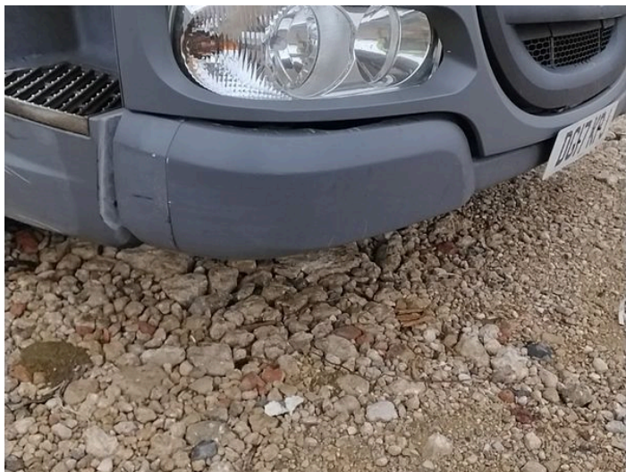
3: Bumper Front Moulding Scuffed (Unpainted) UpTo 100mm
