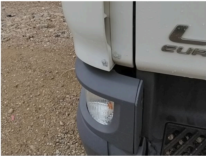
9: Wing nsf Poor Previous Repair Poor Colour
