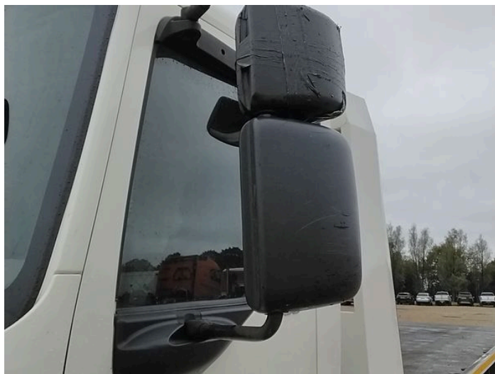
6: Door Mirror Assy nsf Broken Replace
