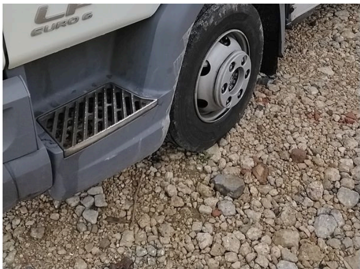
7: Wing Front Arch Extension ns Scuffed (Unpainted) Over 100mm
