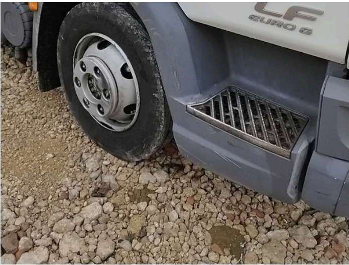
10: Wing Front Arch Extension os Scuffed (Unpainted) Over 100mm
