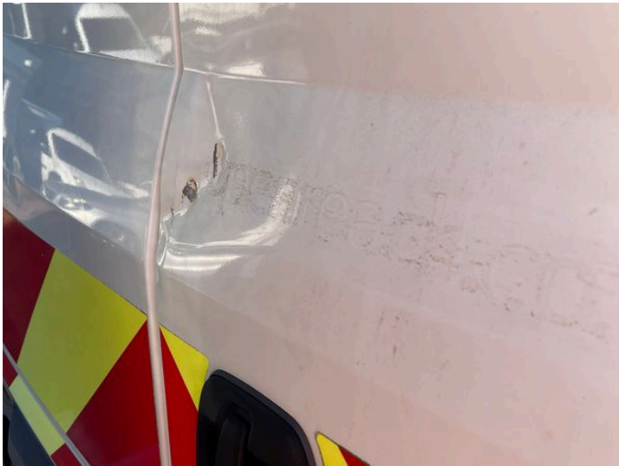
6: Tailgate Dented With Paint Damage
