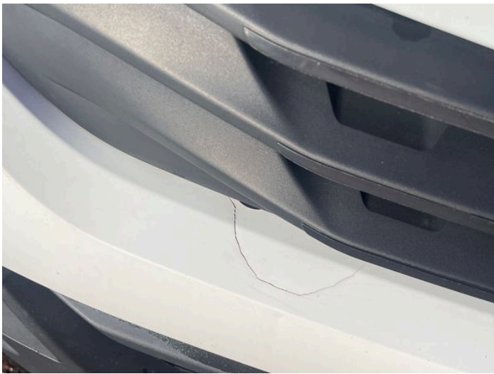
3: Bumper Front Cracked Over 25mm
