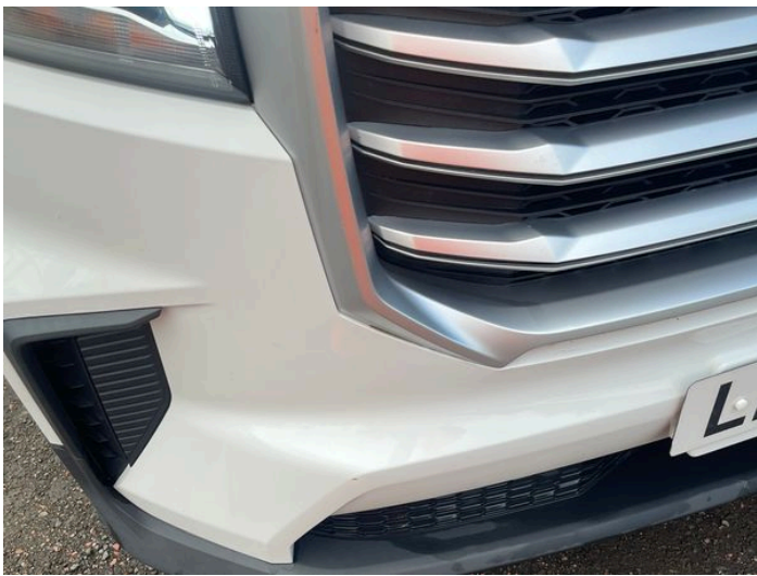
3: Bumper Front Chipped Multiple Chips
