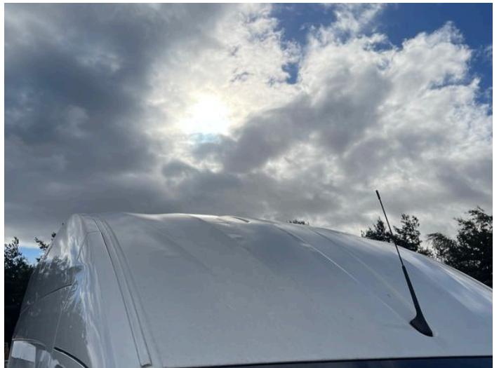
2: Roof Dented With Paint Damage
