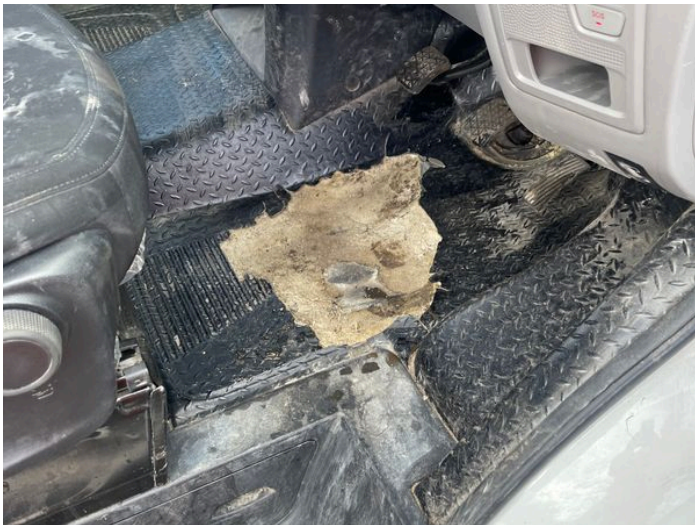
1: Carpets Front Holed Over 3mm
