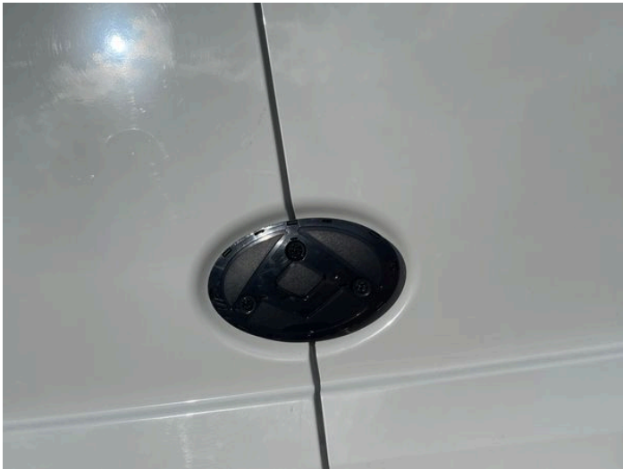
6: Badgedecal Rear Missing Replace
