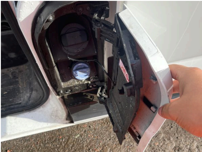
7: Fuel Flap Missing Replace
