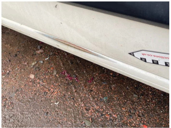
4: Sill os Dented With Paint Damage
