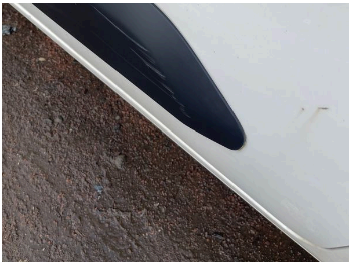
7: Door Moulding nsr Scuffed (Unpainted) Over 100mm
