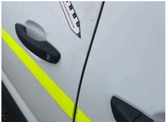
8: Door nsf Dented With Paint Damage
