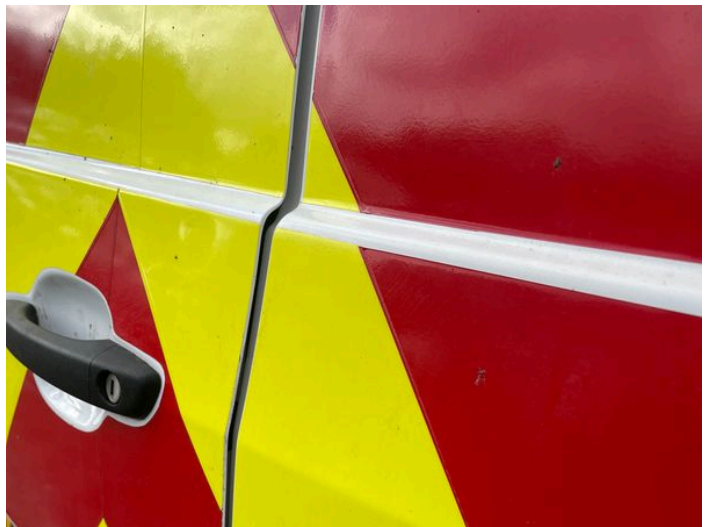
6: Tailgate Dented With Paint Damage
