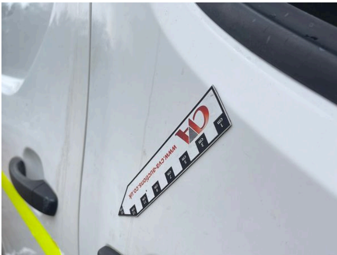
5: Door osf Dented With Paint Damage
