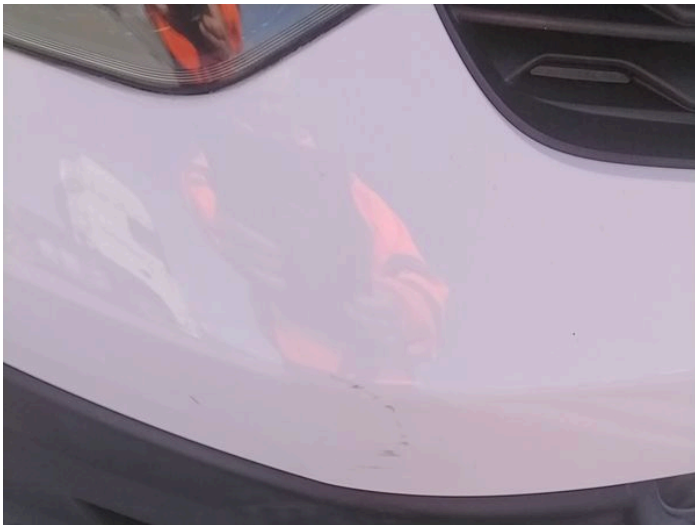
1: Panel Front Scratched Over 25mm Thru Paint
