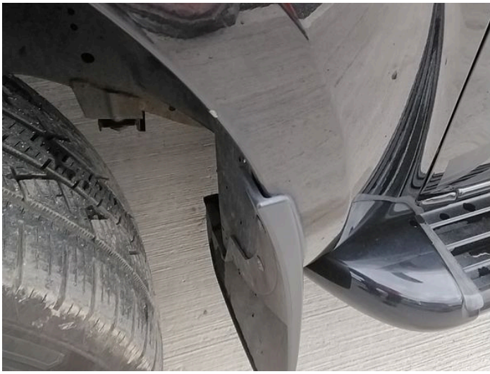
3: Wing nsf Chipped Over 5mm
