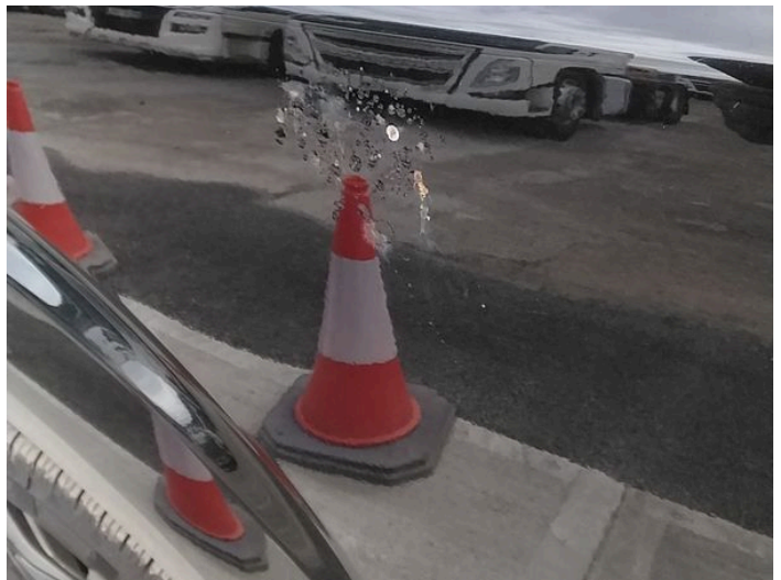
6: Qtr Panel nsr Rusted Over 5mm
