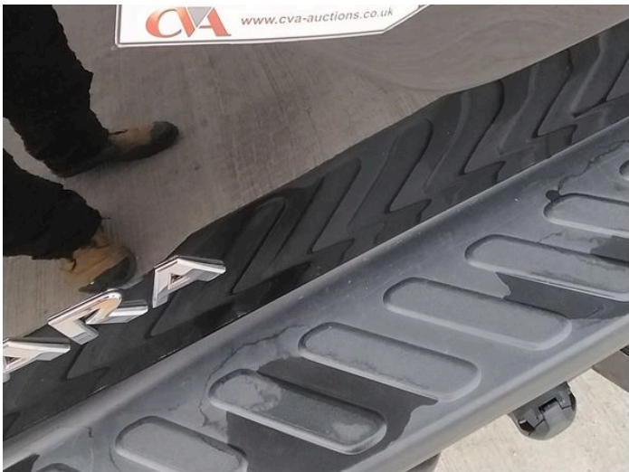
7: Tailgate Scratched Up To 25mm Thru Paint
