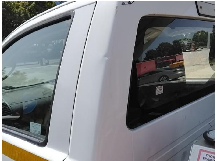
6: B Post ns Rusted Over 5mm
