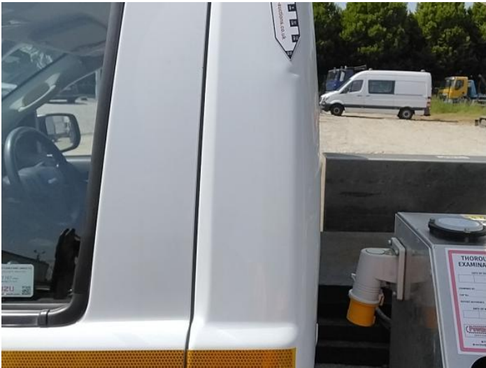
5: B Post ns Dented Over 2 UpTo 10mm
