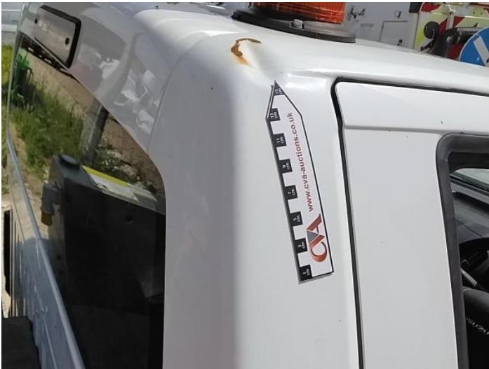
11: B Post os Dented With Paint Damage
