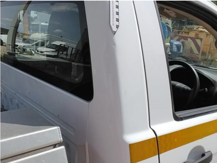
10: B Post os Dented Over 2 UpTo 10mm
