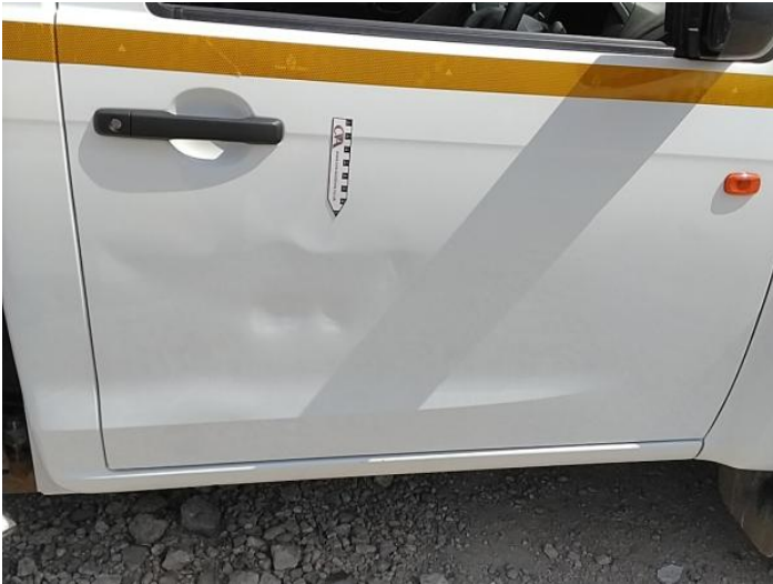
9: Door osf Dented Over 30% Of Panel
