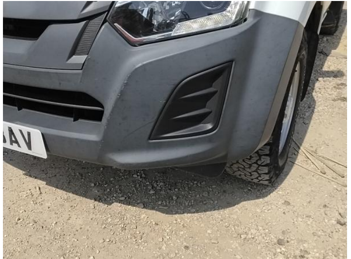
4: Bumper Front Scratched Over 25mm Not Thru Paint
