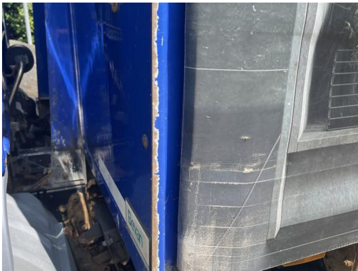
9: Qtr Panel nsr Rusted Over 5mm
