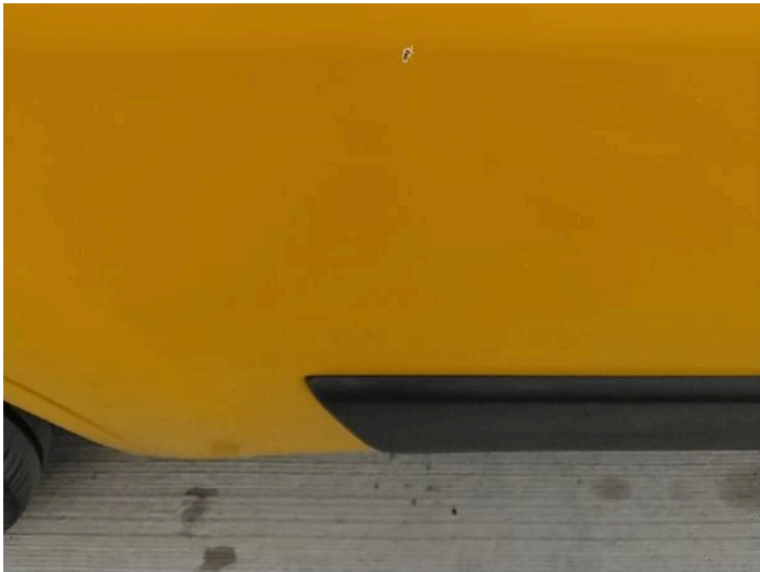
5: Door nsf Chipped Over 5mm
