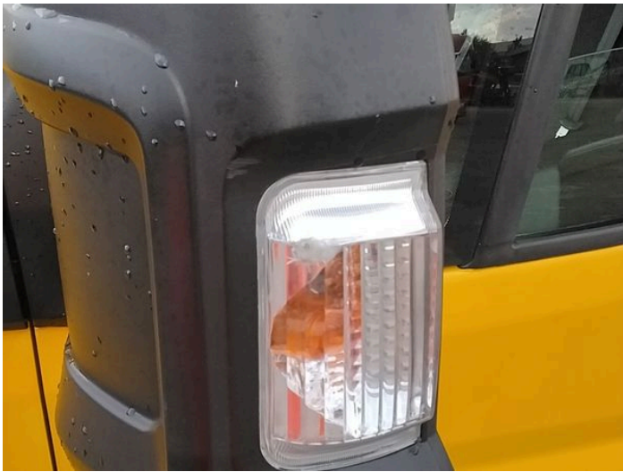
3: Door Mirror Assy nsf Broken Replace
