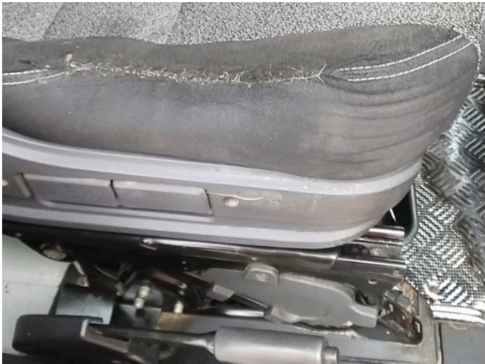
8: Seat Base Cover osf Torn Over 3mm
