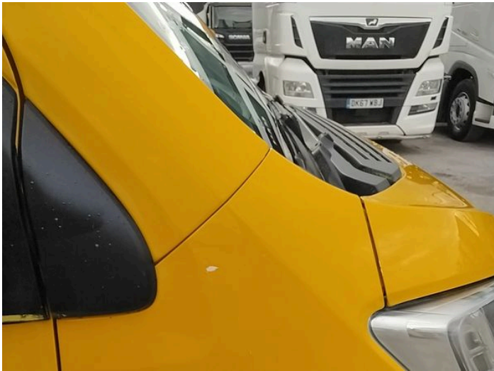
7: Wing osf Chipped Over 5mm
