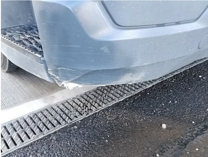
1: Bumper Front Cracked Over 25mm
