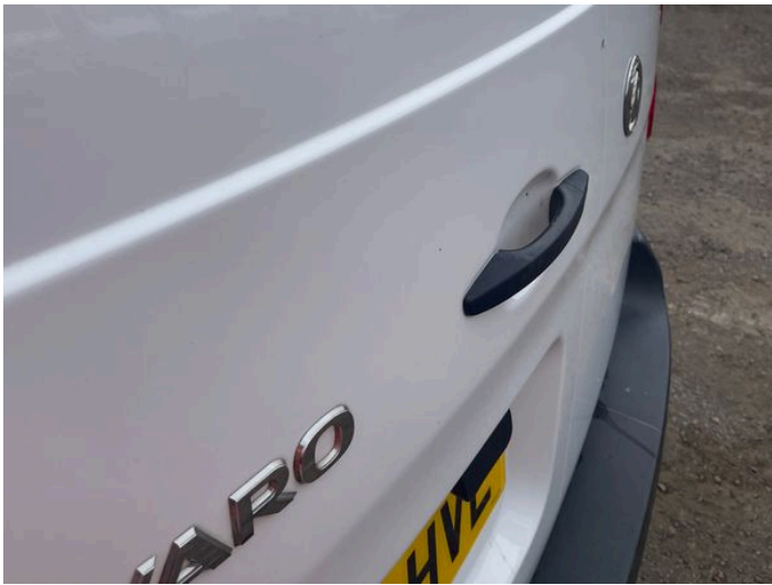
4: Tailgate Dented Over 30mm
