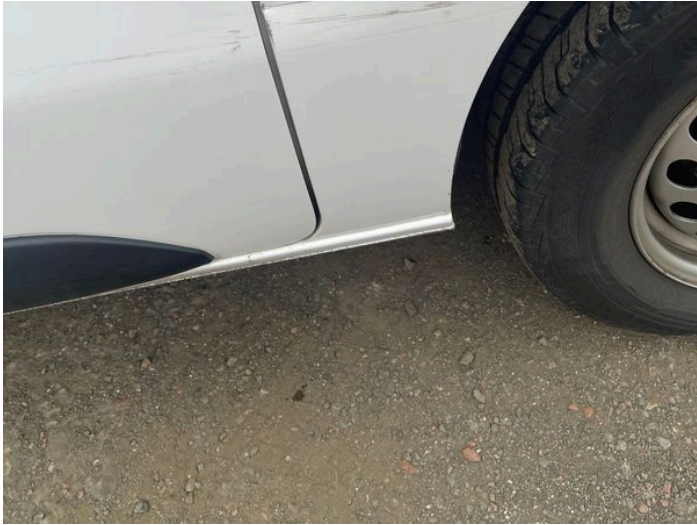
6: Panel Rear Scratched Over 25mm Thru Paint
