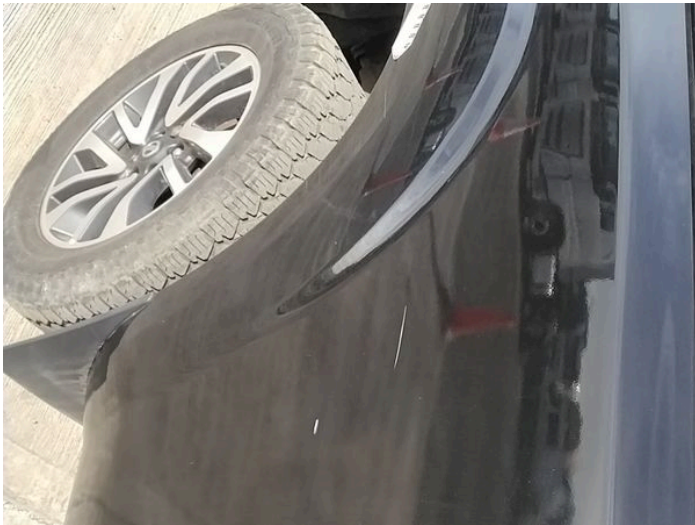
11: Qtr Panel nsr Scratched Over 25mm Thru Paint
