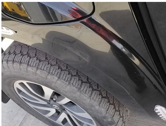
16: Qtr Panel osr Dented With Paint Damage
