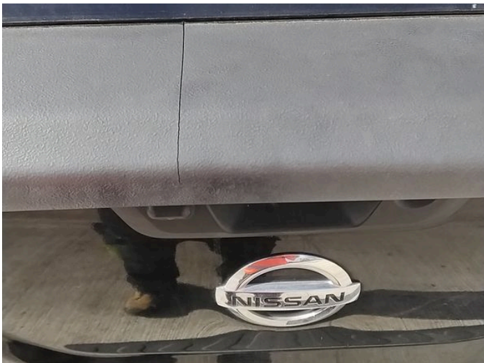
13: Tailgate Trim Panel Broken Replace
