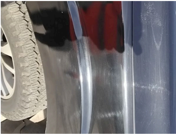
3: Wing nsf Poor Previous Repair Poor Paint
