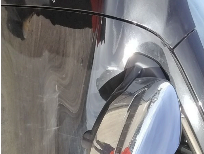
5: Door nsf Scratched Over 25mm Thru Paint
