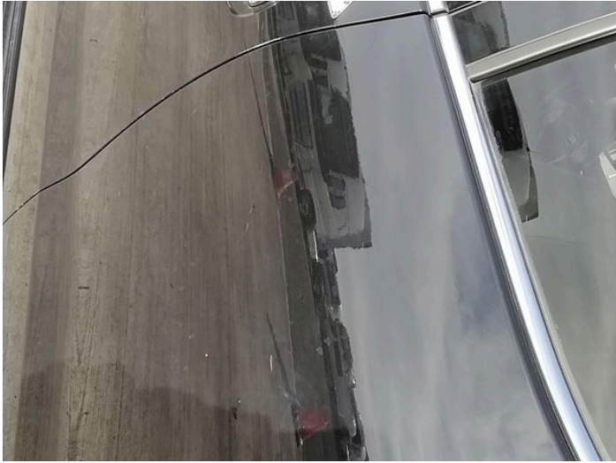
7: Door nsr Scratched Over 25mm Thru Paint
