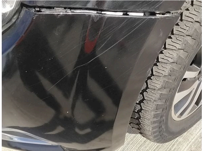
2: Bumper Front Insecure Action Required
