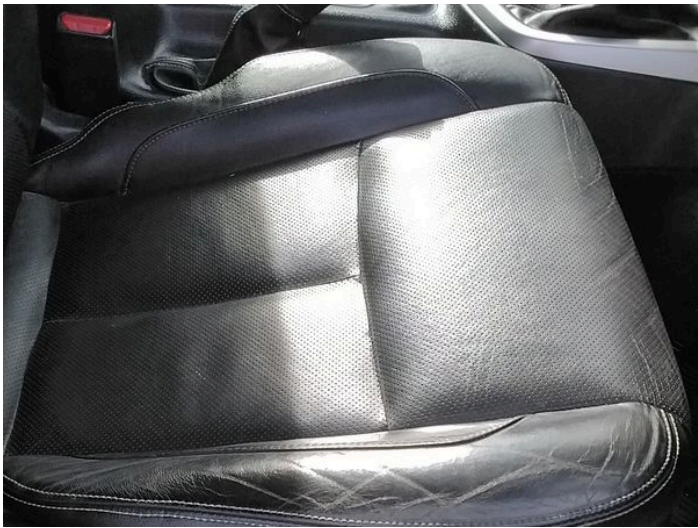
21: Seat Base Cover osf Torn Over 3mm
