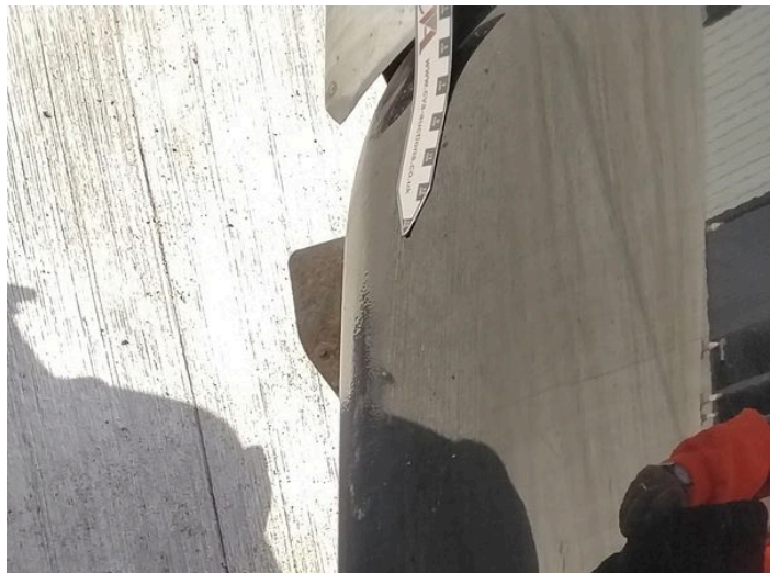
14: Qtr Panel osr Dented With Paint Damage
