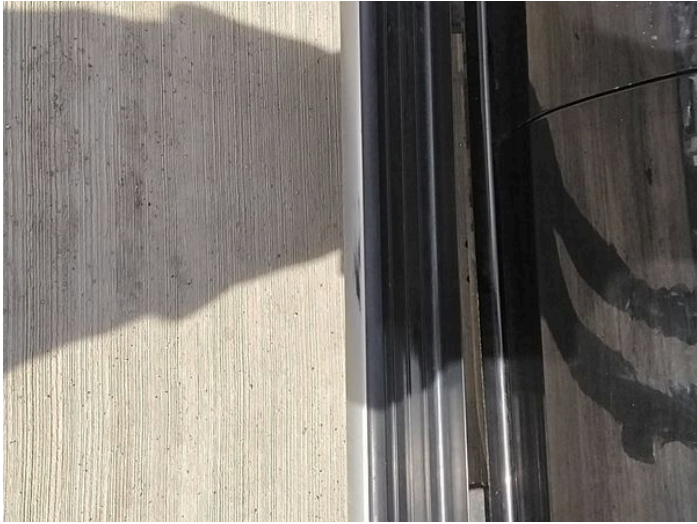
8: Qtr Panel Moulding ns Scuffed (Unpainted) Over 100mm
