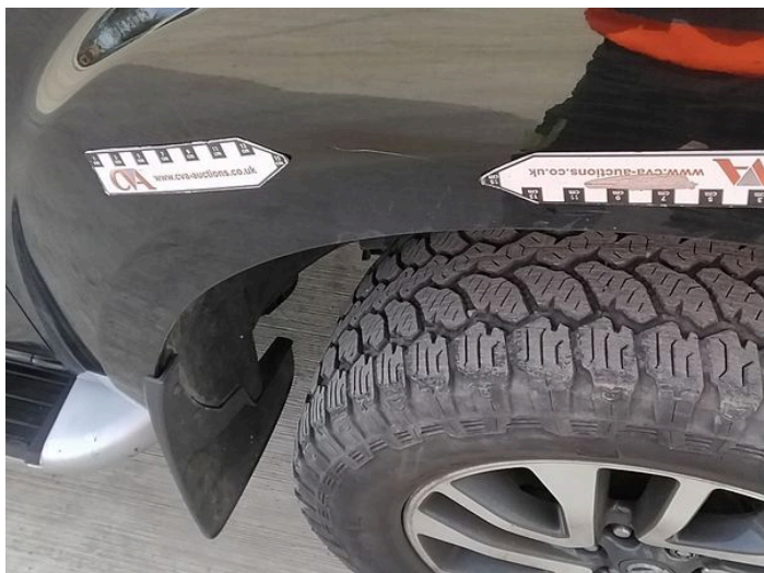
19: Wing osf Scratched Over 25mm Thru Paint
