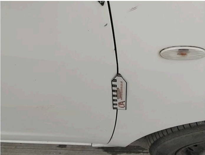
14: Door osf Dented With Paint Damage
