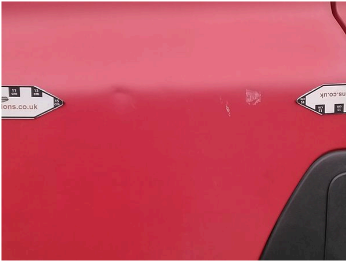
6: Door nsf Dented With Paint Damage
