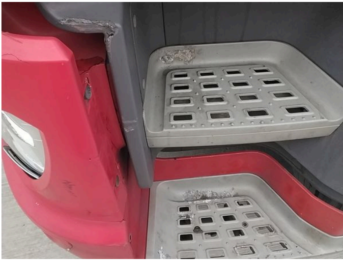
4: Wing nsf Cracked Replace
