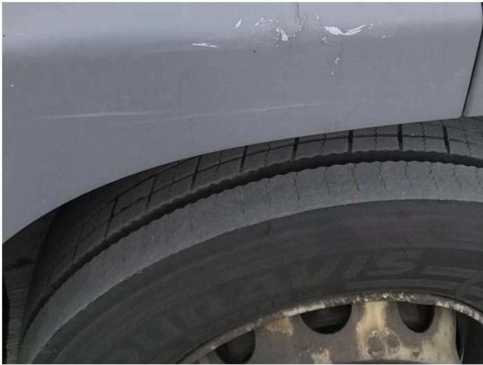
11: Qtr Panel Moulding os Broken Replace
