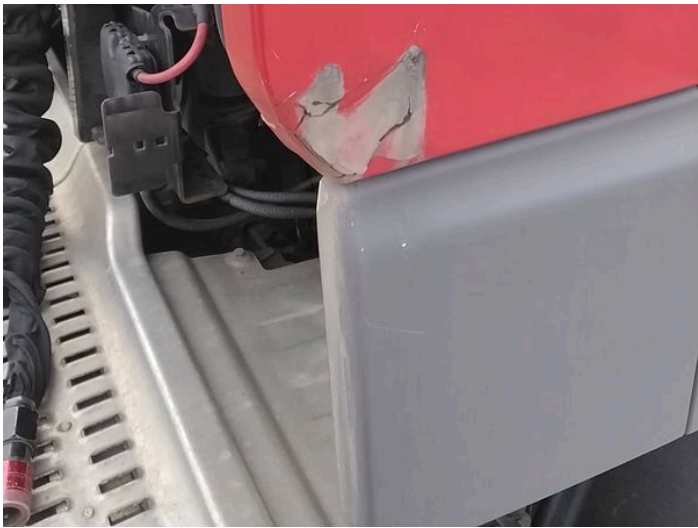
10: Qtr Panel Trim os Broken Replace
