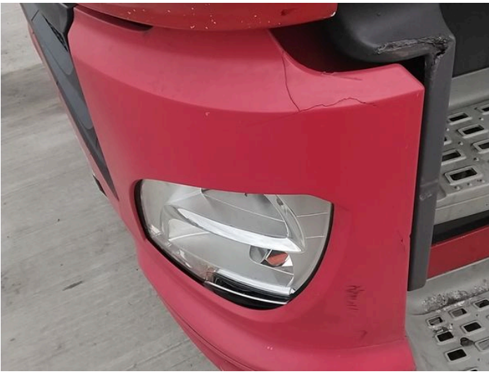
3: Panel Front Cracked Replace
