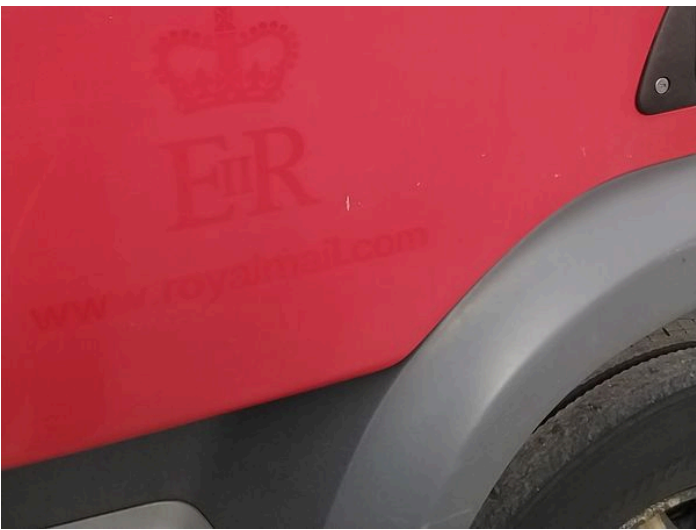
4: Door nsf Chipped Multiple Chips
