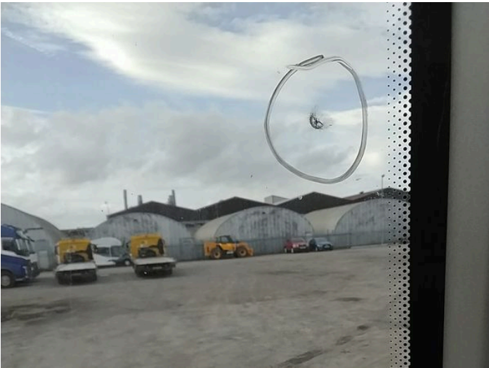
8: Screen Front Chipped Over 10mm
