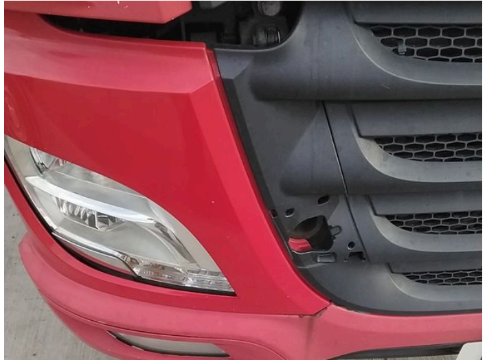
2: Bumper Front Moulding Missing Replace
