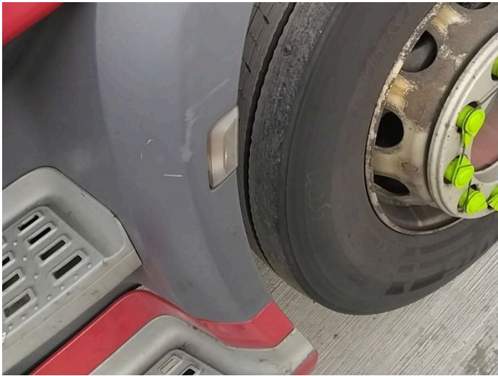
5: Wing nsf Scratched Over 25mm Thru Paint
