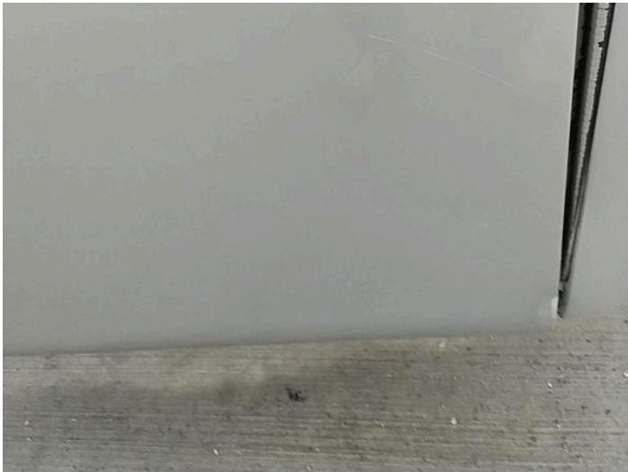
12: Wing osf Scratched Over 25mm Thru Paint
