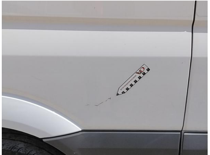
4: Qtr Panel osr Scratched Over 25mm Not Thru Paint
