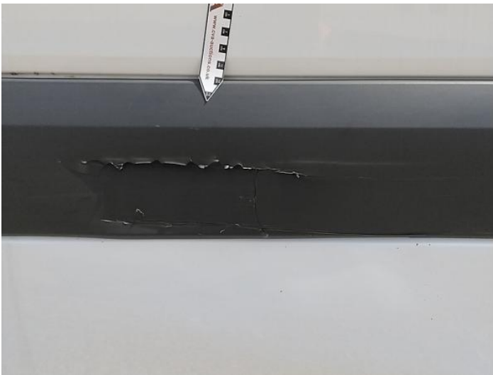
5: Qtr Panel osr Cracked Replace
