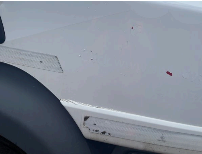
3: Door osf Chipped Multiple Chips
