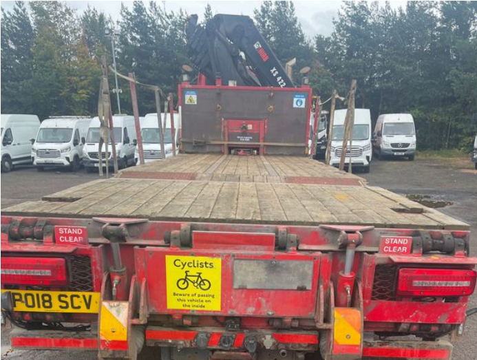
5: Tailgate Rusted Over 5mm
