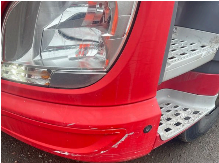
8: Qtr Panel Moulding ns Scratched (Painted) Over 25mm Thru Paint
