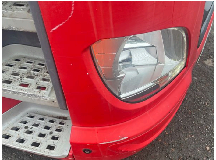
2: Qtr Panel Moulding os Scratched (Painted) Over 25mm Thru Paint
