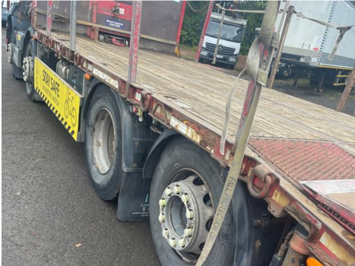
6: Qtr Panel nsr Rusted Over 5mm
