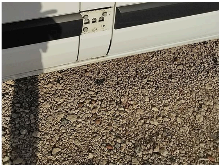
9: Qtr Panel Trim ns Missing Replace
