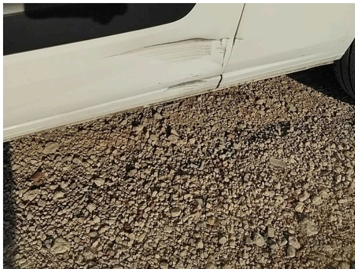
10: Door nsr Dented With Paint Damage
