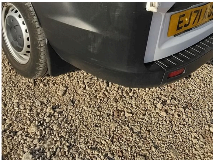
11: Bumper Rear Moulding Scuffed (Unpainted) Over 100mm
