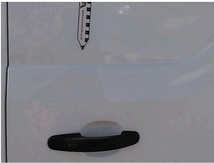
15: Door osr Dented Between 10mm + 30mm
