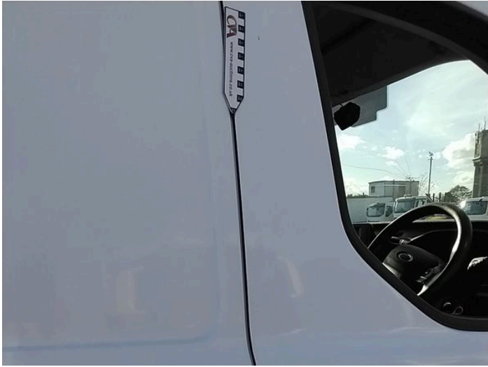
19: Door osf Chipped Edge Chip
