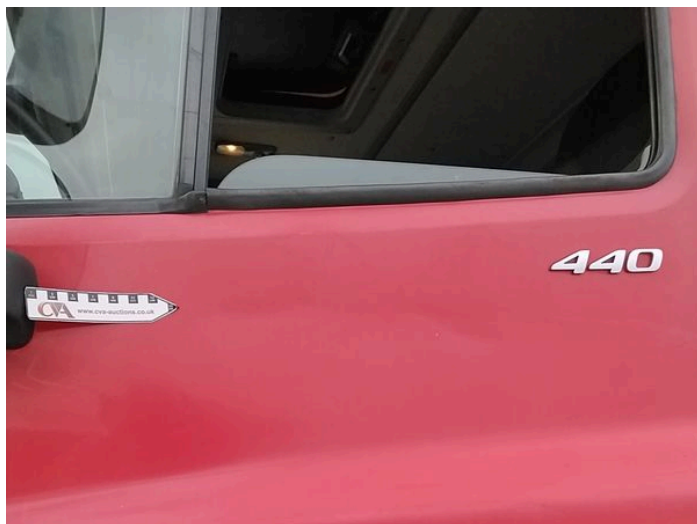
8: Door nsf Dented Over 30mm
