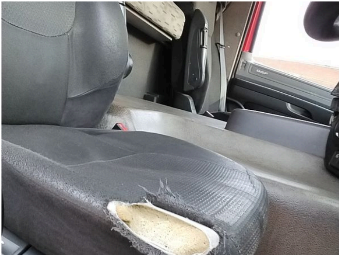
12: Seat Base Cover osf Holed Over 3mm
