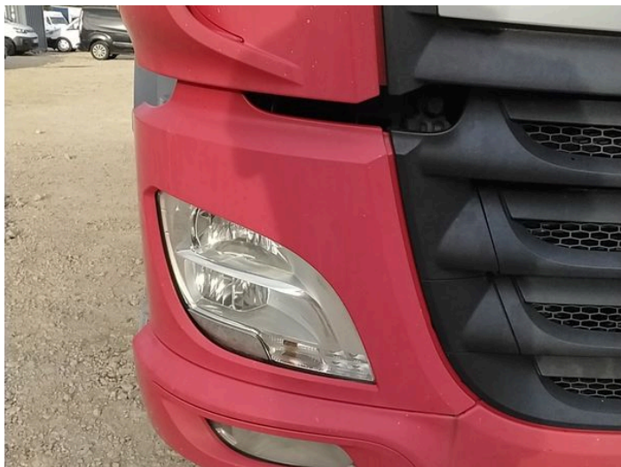
3: Fog Lamp Surround os Scratched (Painted) UpTo 25mm Thru Paint
