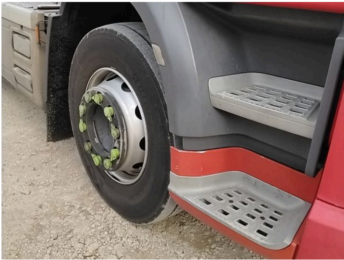
10: Wing Front Arch Extension os Scuffed (Unpainted) UpTo 100mm
