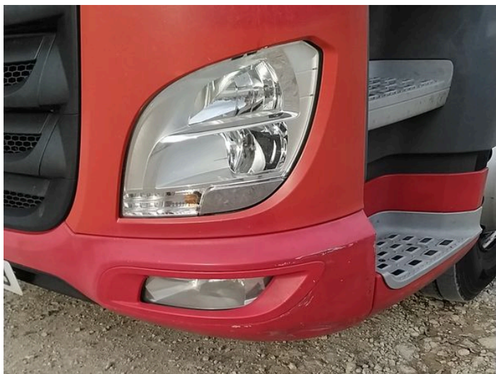
5: Bumper Front Dented With Paint Damage
