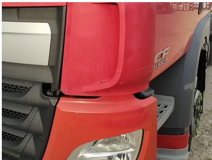
6: Wing nsf Cracked Replace
