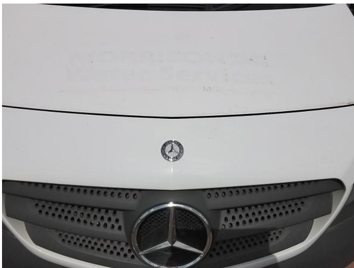
1: Bonnet Chipped Multiple Chips
