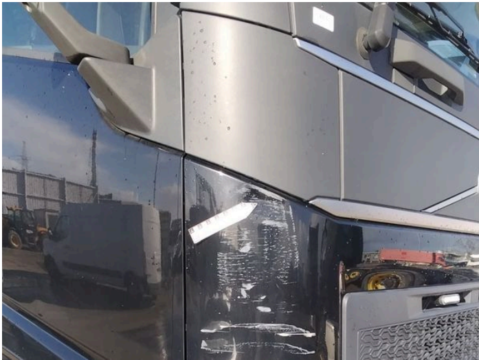
13: Wing osf Dented Over 30mm
