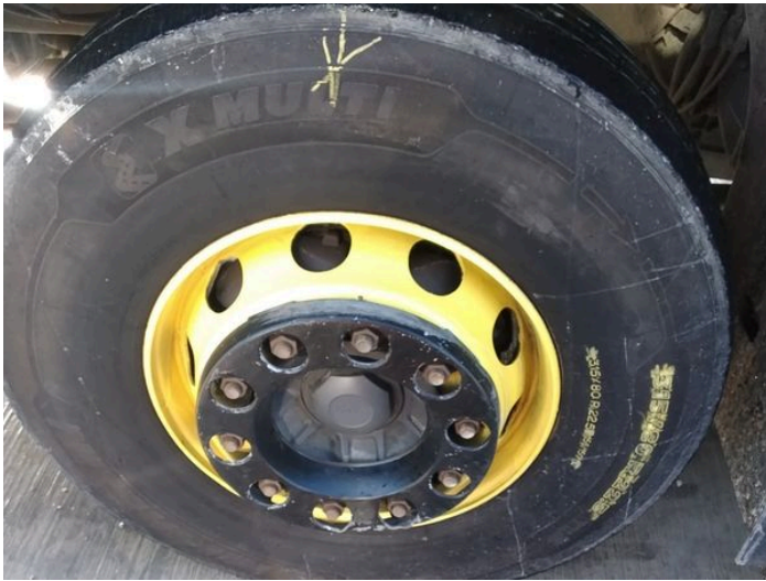
5: Wheel nsf Corroded Light
