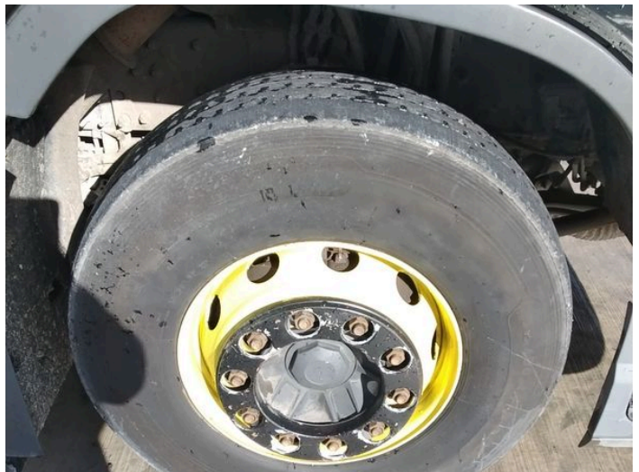
8: Wheel osf Corroded Light
