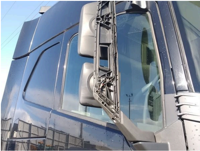
12: Door Mirror Assy osf Missing Replace
