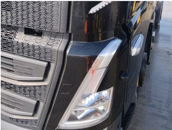
1: Wing nsf Scratched Over 25mm Thru Paint
