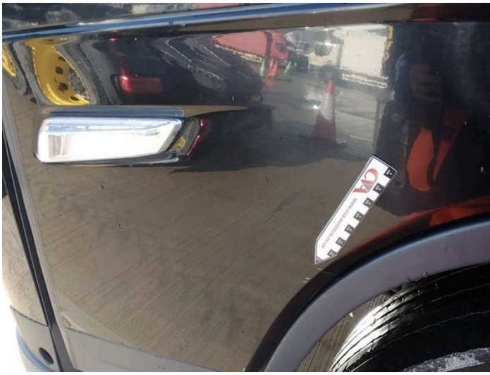
3: Door nsf Scratched UpTo 25mm Thru Paint
