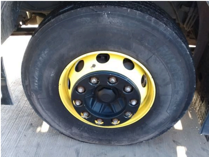
7: Wheel nsf Corroded Light
