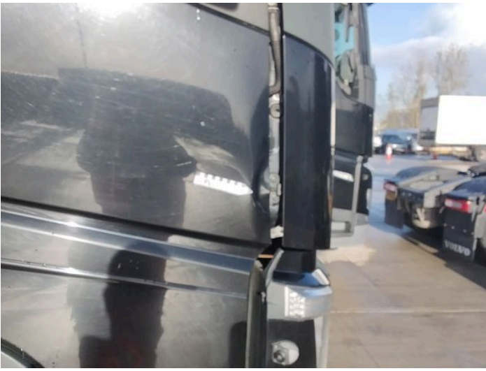
15: Door osf Dented Over 30mm
