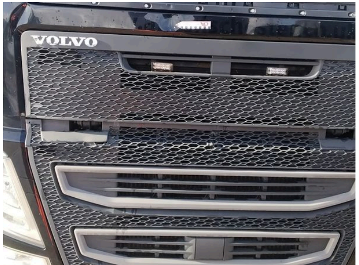
2: Panel Front Dented Over 30mm
