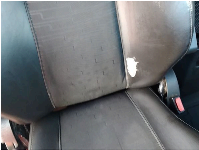
21: Seat Back Cover osf Torn Over 3mm
