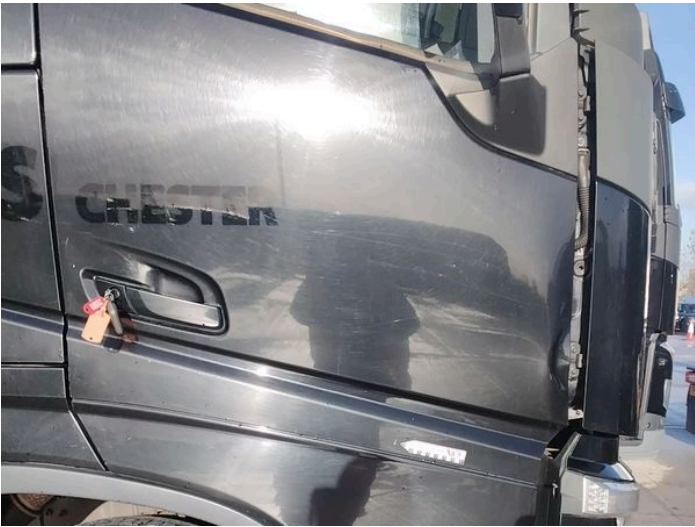
17: Door osf Chipped Over 5mm
