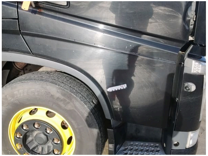
16: Door osf Scratched Over 25mm Thru Paint
