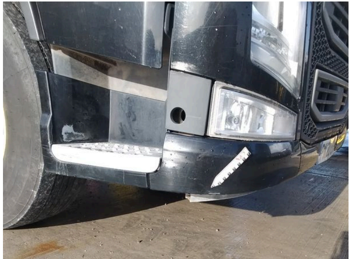
20: Bumper Front Scratched Over 100mm Thru Paint
