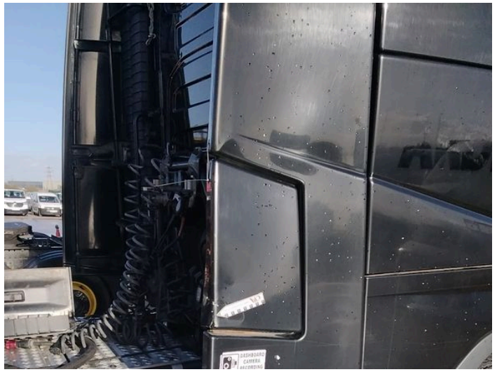
10: Qtr Panel osr Cracked Replace
