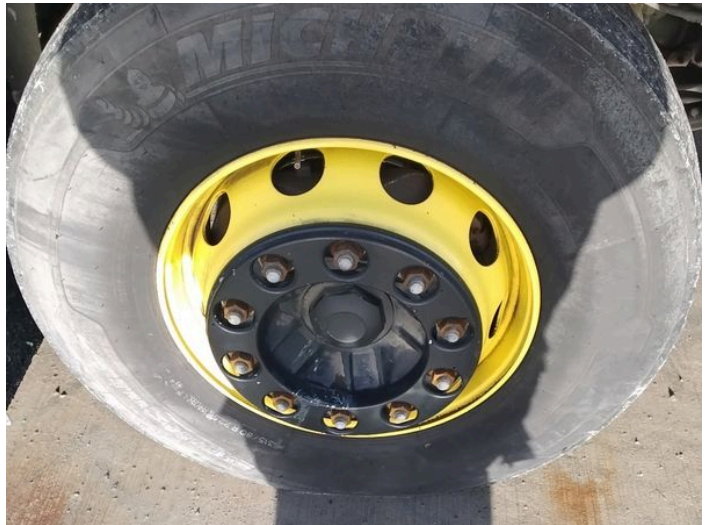
12: Wheel osf Corroded Light
