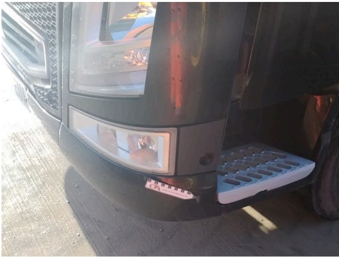
4: Bumper Front Scratched Over 100mm Thru Paint
