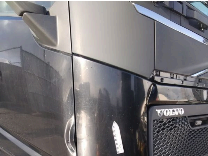
19: Wing osf Scratched Over 25mm Thru Paint
