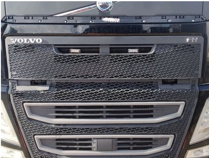
1: Panel Front Missing Replace
