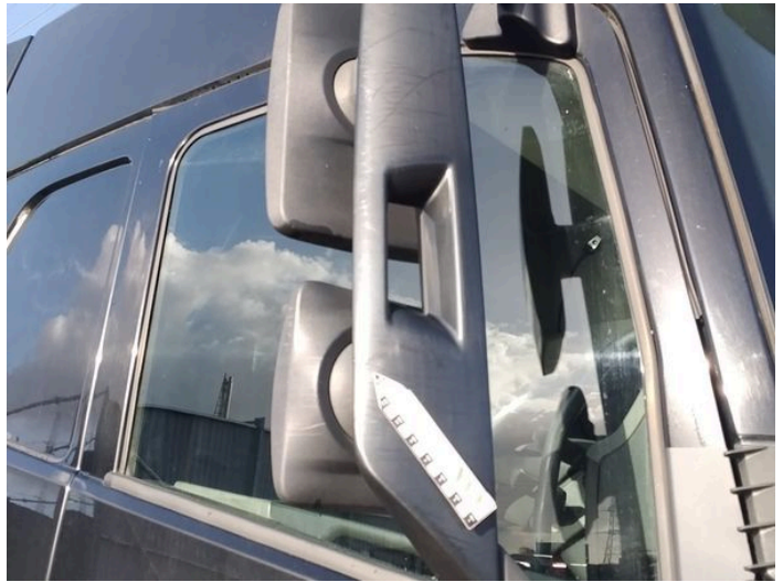
18: Door Mirror Assy osf Scuffed (Unpainted) Over 100mm
