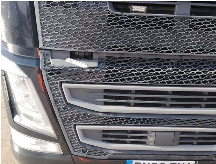
3: Grille Front Broken Replace
