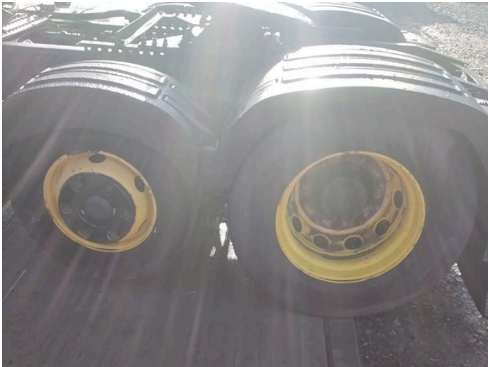
8: Wheel nsr Corroded Light
