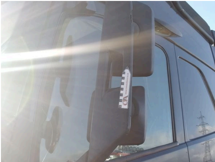
5: Door Mirror Assy nsf Broken Replace
